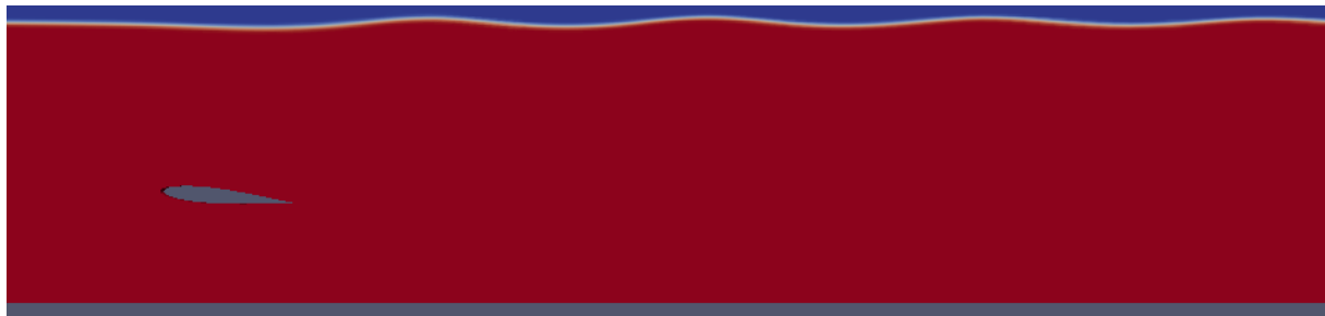
Figure 7-2: Simulation of the surface in paraView. Result obtained from mesh3, with interFoam solver. Red represent water, blue air, with a thin interface inbetween.
