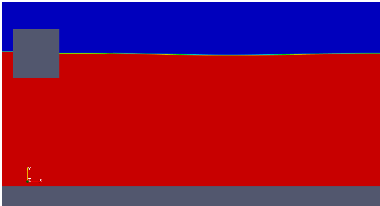
Figure 7-11: Overview of the generated waves, and the free surface. Red is water, blue is air, and between is the interface.
