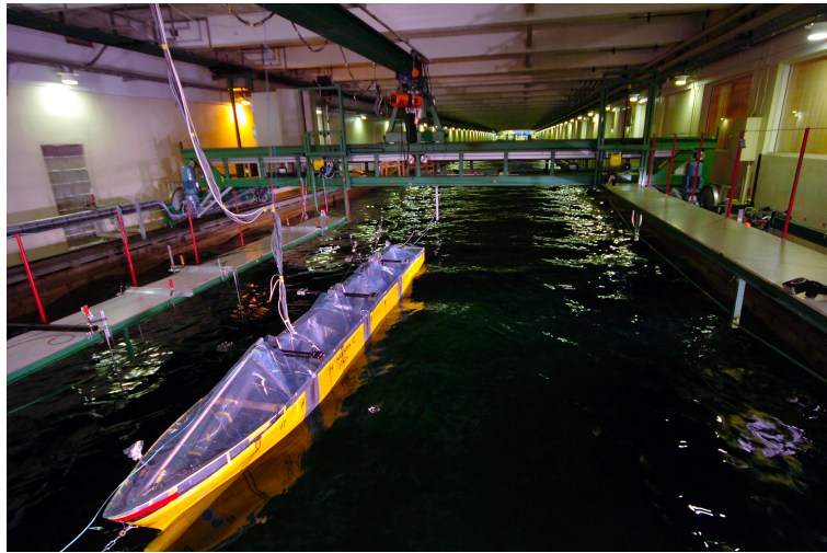
Figure 3.26: Picture of the model under the carriage in the towing tank.
