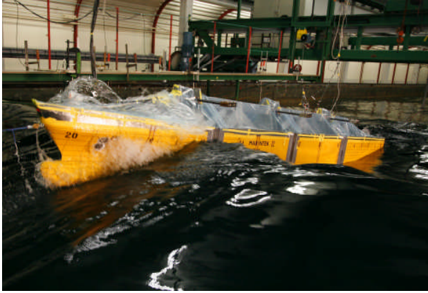
Fig. 2: Model and Towing Carriage
