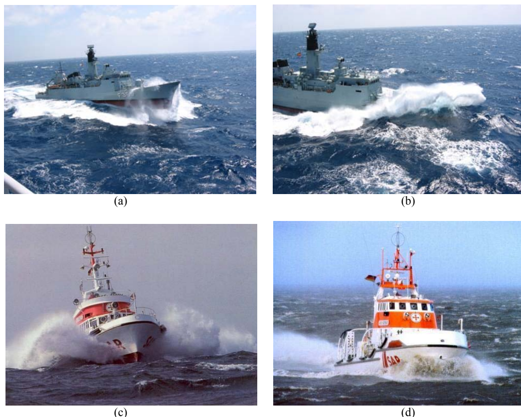
Fig. 1.2. Examples of slammings on ships. (a) Bottom slamming; (b) Green water slamming; (c) Bow-flare slamming; (d) Bow stem slamming (Photos downloaded from the internet).
