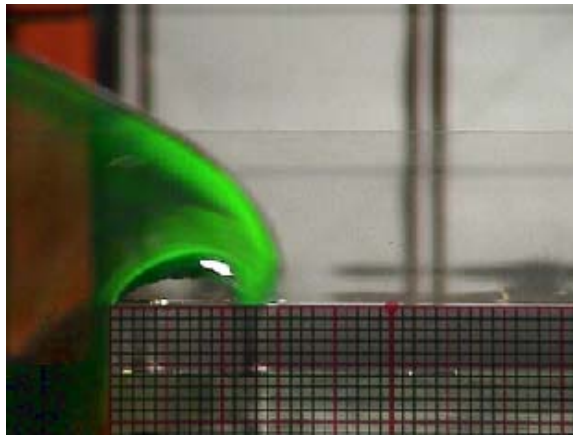
Figure 7.4 The initial phase of water on the deck of a 2D ship-like body that was restrained from oscillating. A plunging wave impacts against the deck and an air cushion is created (Greco, 2001).
