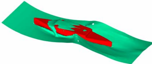
Figure 7.3 3D water-on-deck simulations for a Wigley hull in regular head sea waves with wave height-to-wavelength ratio 0.1 and wavelength-to-ship length ratio 1.0. Fn=0.25 . T_w =wave period.
