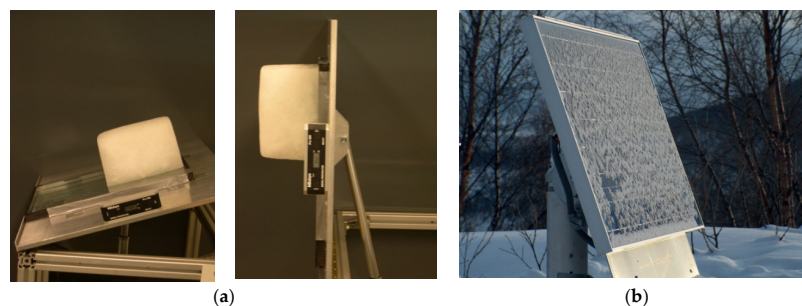
Figure 23. A snow/ice slab firmly sticking to the glass surface of an insulated window pane even at an inclination angle of 90^\circ during a laboratory experiment (a). Snow covering a solar cell panel at an inclination angle of 70^\circ (b) [173].
