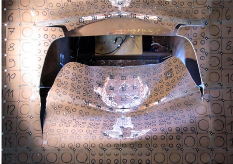
(a) Experimental failure mode, figure from Fricke et al. (2014)
