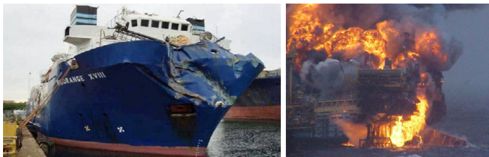
(a) Damage to Big Orange after impact to Ekofisk jacket (b) Mumbai High North on fire
