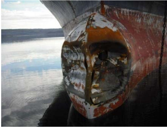
Figure 7.1: Bow damage from ice action to a 1A-classed vessel, June 2012, from Canadian Coast Guard (2012)
