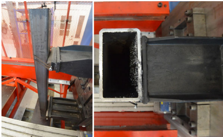
Figure 8.14: Hollow profile beam mounted on two simple supports. Rubber bands attach the beam to the supports.
