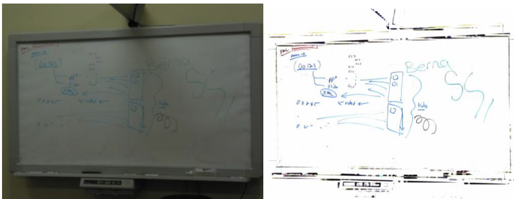
Figure 3: (left) Whiteboard image captured by a digital camera (right) enhanced with the Gormish et al. method [19]
