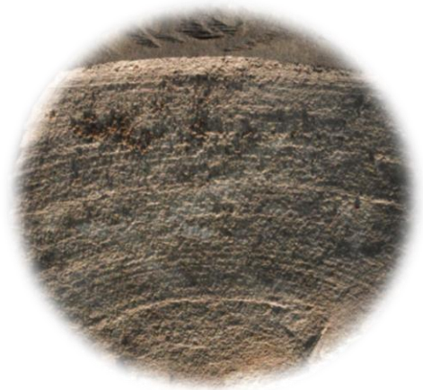
Figure 8.1: Beach marks on a fatigue fracture surface. The crack originates from the center of the rings. Taken from Fontenot W, Zhang L. 76 mm Chain Link Fatigue Failure. SOFEC Inc., Stress Engineering Services Inc. [undated; 27.04.2014]
