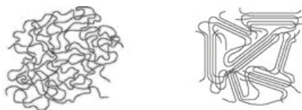
Figure 2.1: Amorphous (left) and semi-crystalline (right) arrangement of polymer molecules.
