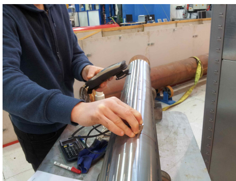
Figure A.2: Wall thickness measurement with a ultrasonic thickness gage.
