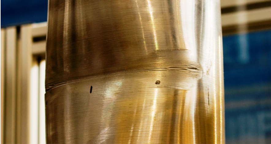
Figure 3.12: Surface fracture observed on pipe A, exposed to both dynamic impact and stretching. This pipe was impacted with a trolley velocity of 3.24 m/s, with mass equal to 1472kg [37].
