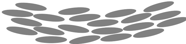
Figure 1.1: Illustration of the orientational ordering in nematic liquid crystals. The elongated molecules tend to align their long axes while flowing like a liquid.
