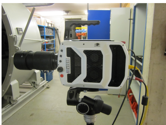
(c) High-speed camera operating at 75 000 fps.
