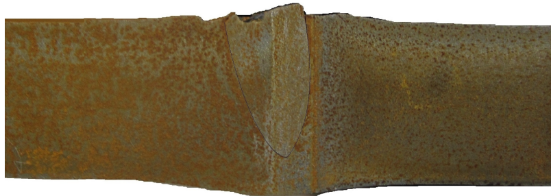
(a) 12 mm Test no. 3. v_i = 466.90 m/s.
