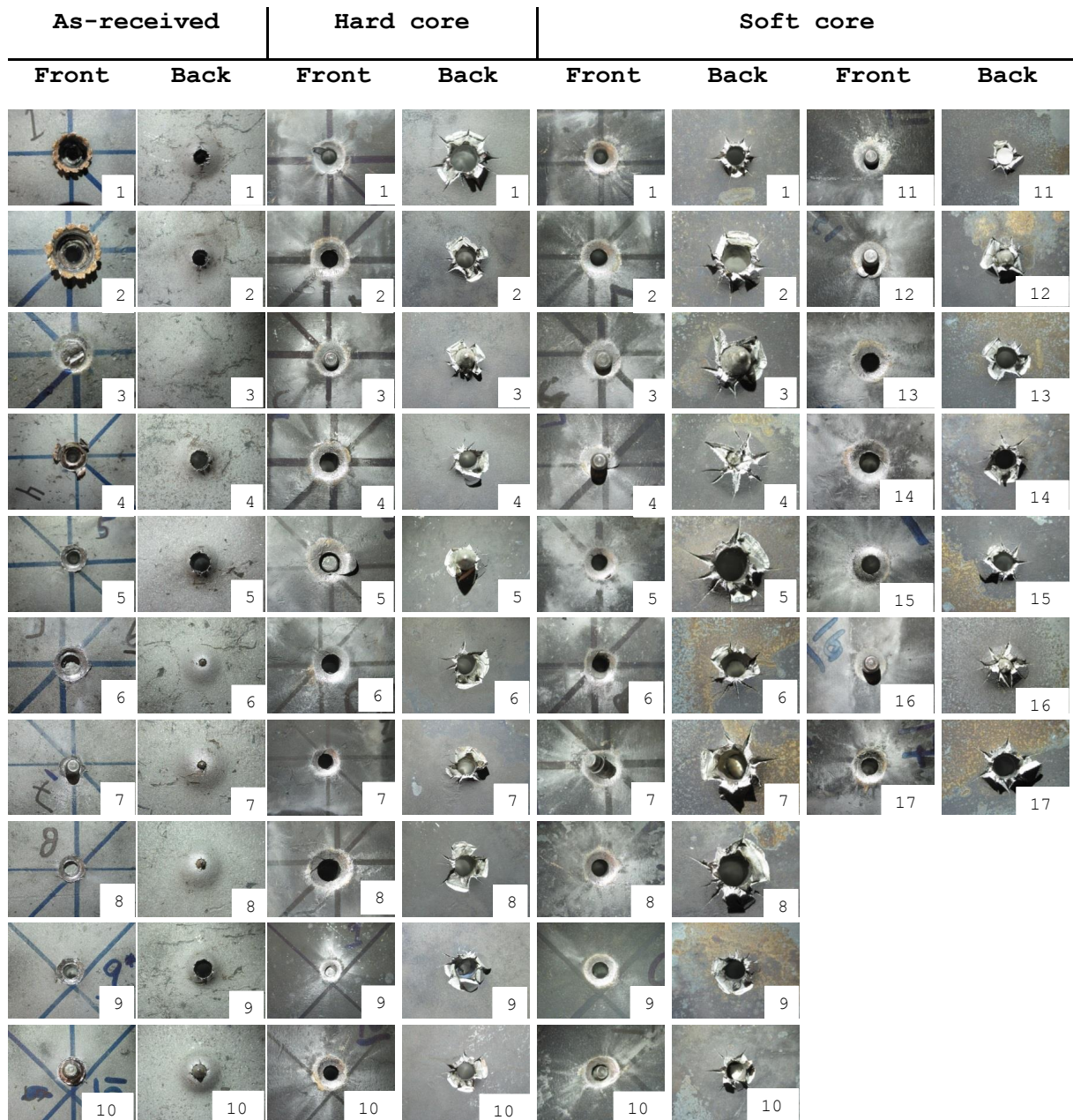
Figure A.1: Bullet holes - 12 mm plates.
