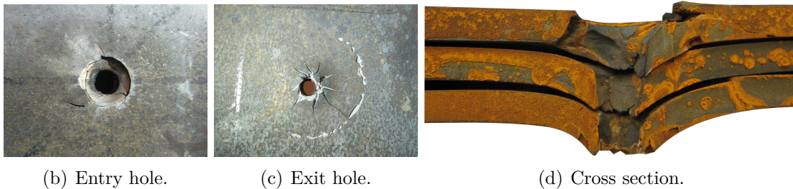
Figure 4.14: Test no. 1 for soft core 3x4 mm plate. v_i=916.00 m/s, v_r=550.90 m/s.
