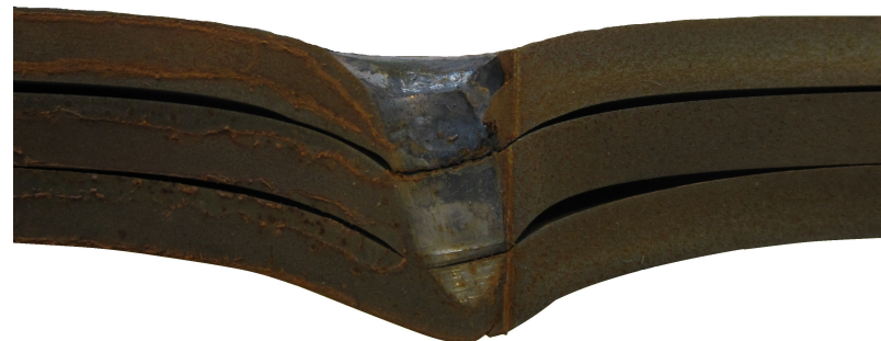
(c) 4x4 mm Test no. 7. v_i = 570.80 m/s.
