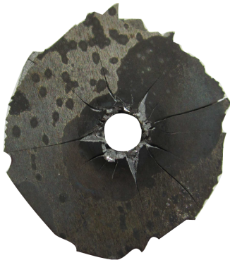
(c) Test no. 2: Back plate halo.
