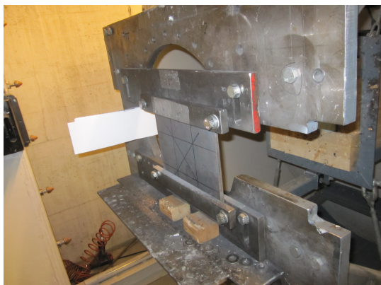
(a) Target plates clamped to rigid frame by transverse beams.
