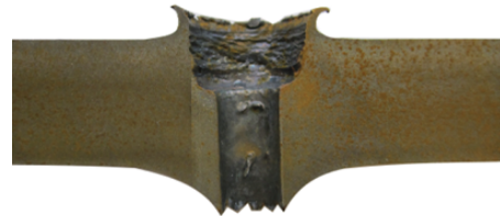
(b) Experiment: v_i=745.10 m/s, v_r=500.60 m/s.
