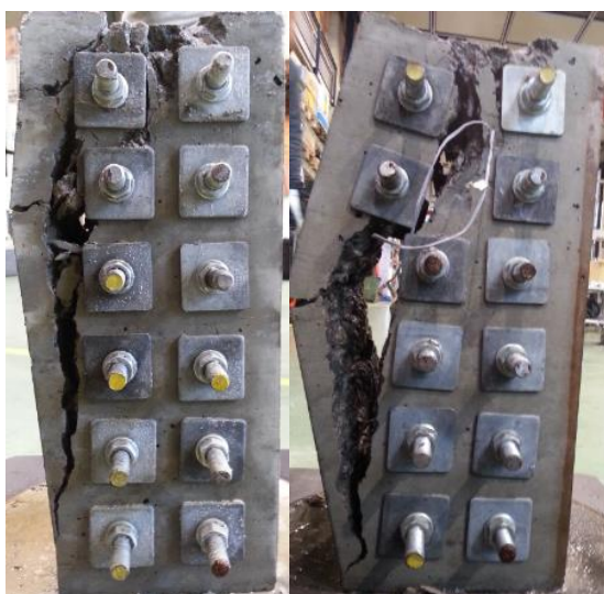
Figure 74 - Crack at failure in reinforced (left) and unreinforced (right) specimens
