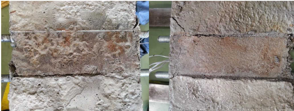
Figure 60 – Short term specimen 9 unreinforced (left) and short term specimen 15 reinforced (right)
