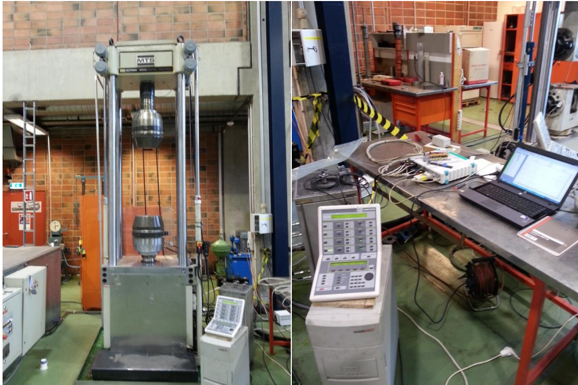
Figure 20 - Hydraulic jack "MTS", Instron 8500 controller, Spider8 logger and a computer
