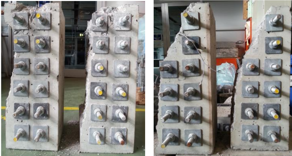
Figure 75 - Crack at failure (disassembled) in reinforced (left) and unreinforced (right) specimens
