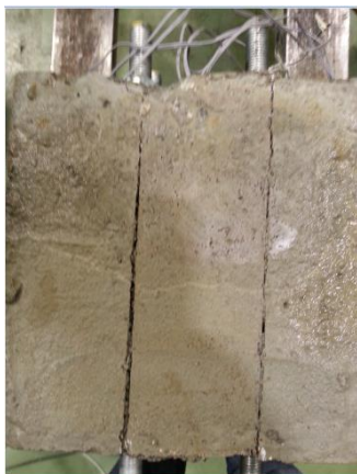
Figure 40 - Crushing of the top in static specimens
