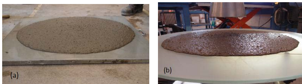
Figure 2-8 Mix 4 (a) before fiber addition (b) after fiber addition
