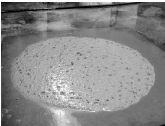
FIG. X1.3 VSI = 2 - Evidence of a Mortar Halo and Water Sheen.
