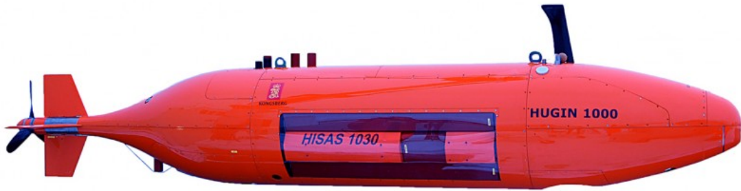
Figure 1. HUGIN 1000 AUV with HISAS (HISAS 1030, two on each side of vehicle) (Geomares Publishing bv, 2012 - 2015).
