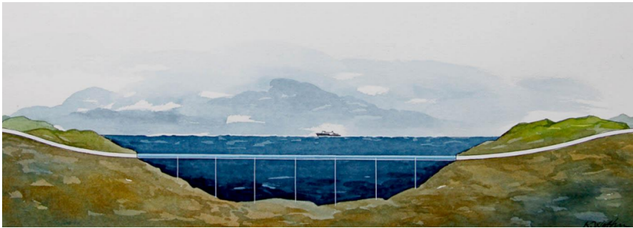
Figure 1: The submerged floating tunnel concept (NPRA, 2012)
