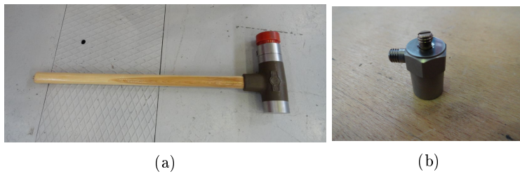
Figure 4.9: The modal hammer (a), and the accelerometer (b)
