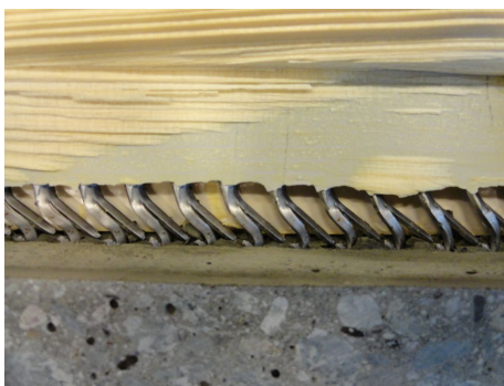
Figure 7.1: The failure mode of the shear connector
