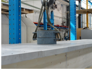
Figure 4.12: The weights applied in load case 3
