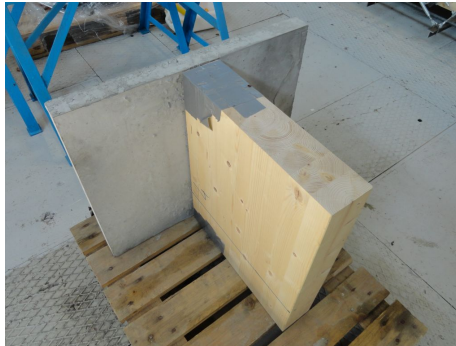
Figure 4.7: The shear test specimen
