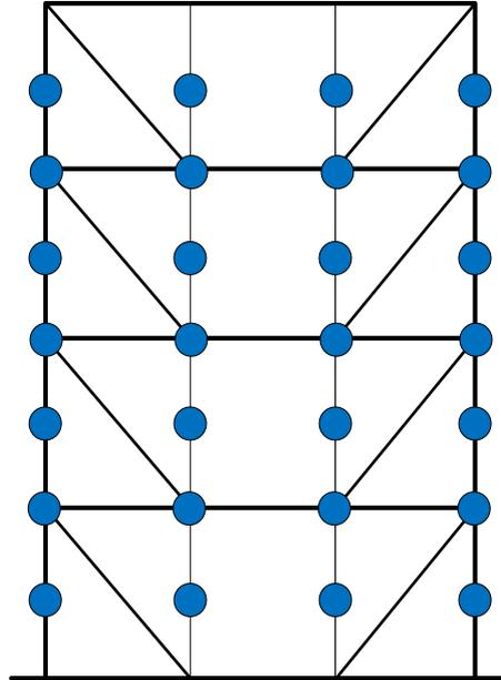
FIGURE 57: LOAD POINTS ON FRAME
