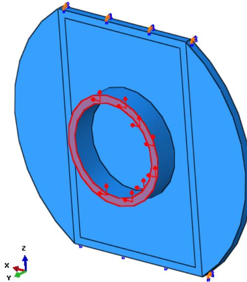
FIGURE 84: LOAD AT REAR TRUNNION
