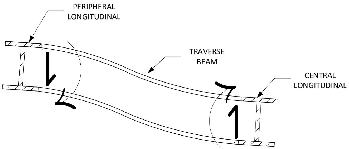
**FIGURE 59: BENDING OF TRAVERSE BEAMS COUNTERING HEIGHT DIFFERENCE OF CENTRAL AND PERIPHERAL LONGITUDINALS**
