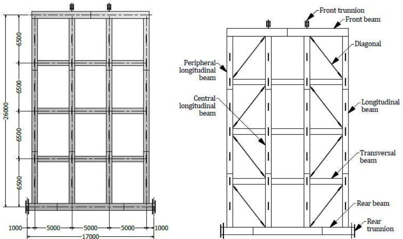
FIGURE 34: GEOMETRY DIMENSIONS AND MEMBER ANNOTATION
