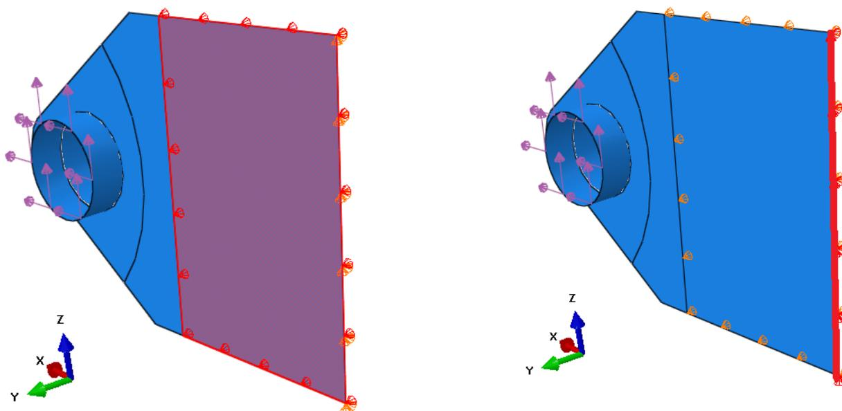
Red area restrained toward translation in y-direction (out-of-plane deformation)
