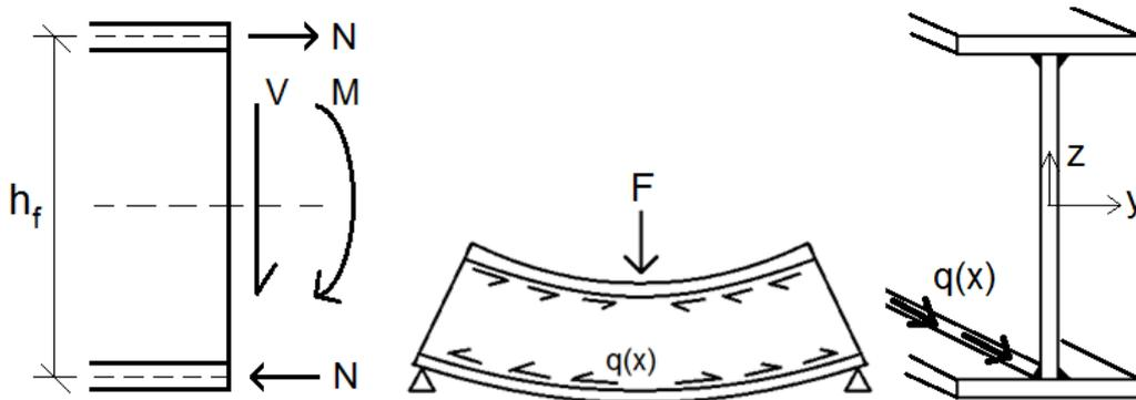
FIGURE 69: FORCES IN CROSS SECTION AND SHEAR FORCE IN WELDS
