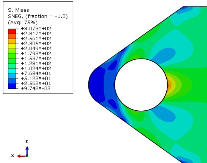
FIGURE 91: STRESS AND DEFORMATION OF FRONT TRUNNION IN 1) HORIZONTAL POSITION
