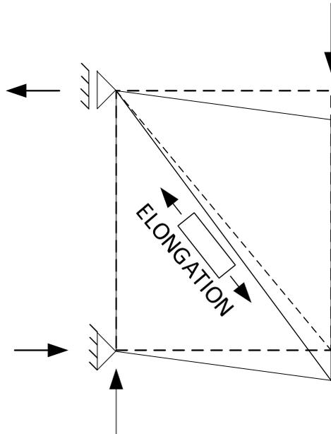
**FIGURE 65: WEIGHT TRANSMISSION THROUGH DIAGONALS**
