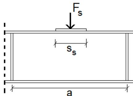
FIGURE 73: CALCULATION MODEL FOR PLATE RESISTANCE TO TRAVERSE FORCE
