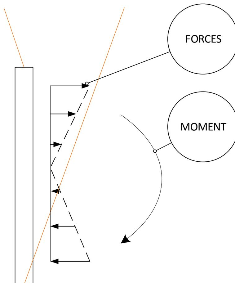
FIGURE 63: MOMENT AND RESULTING HORIZONTAL FORCES
