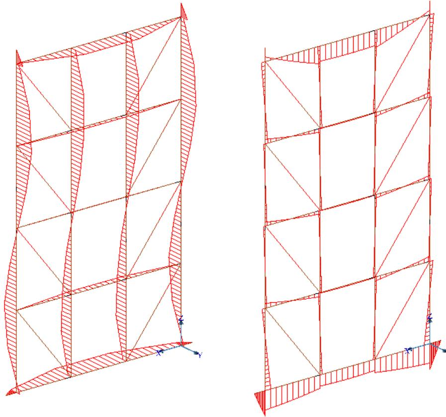
FIGURE 99: FORCES IN VERTICAL POSITION: LEFT - AXIAL FORCE, RIGHT - MOMENT ABOUT STRONG AXIS
