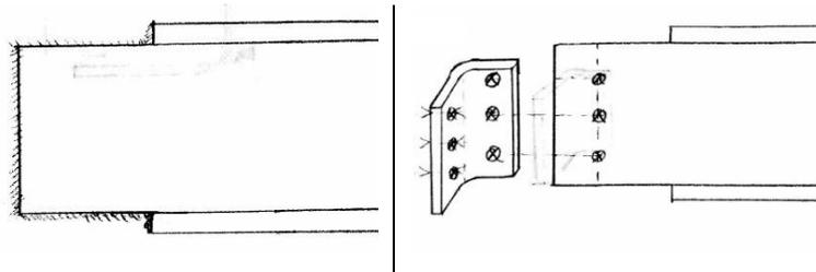
FIGURE 18: WELDED AND BOLTED JOINT OF I/H BEAMS
