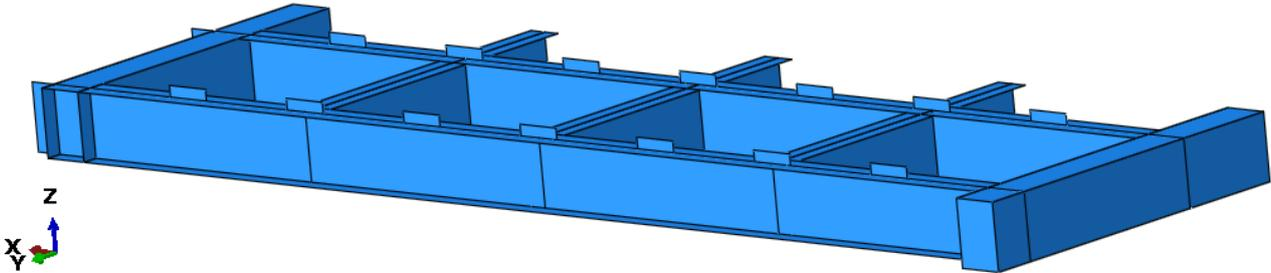
FIGURE 78: SHELL MODEL OF THE FRAME
