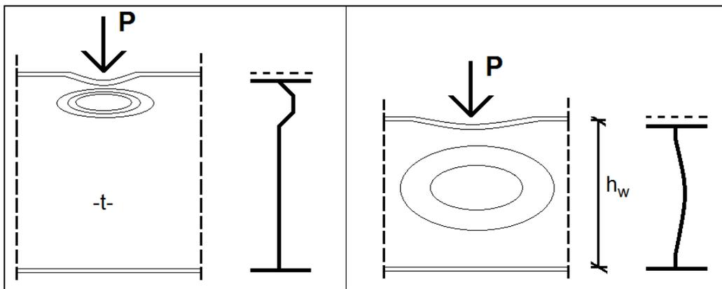
FIGURE 72: BUCKLING OF PLATE DUE TO TRAVERSE FORCE
