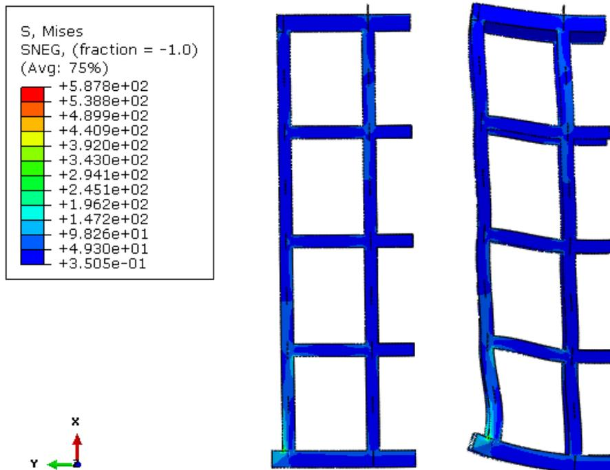
FIGURE 88: STRESS DISTRIBUTION AND DEFORMATION IN VERTICAL POSITION
