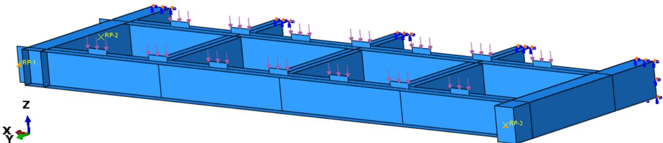
FIGURE 79: SHELL MODEL WITH LOADS AND BOUNDARY CONDITIONS
