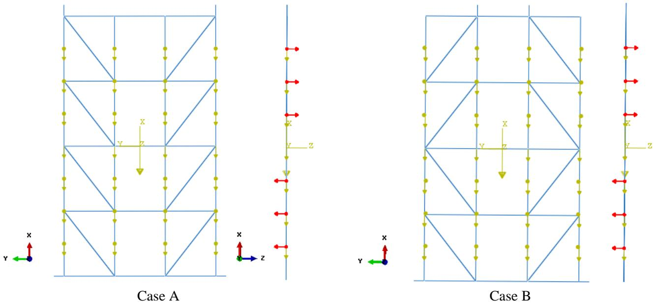
FIGURE 76: LOADS IN VERTICAL POSITION
