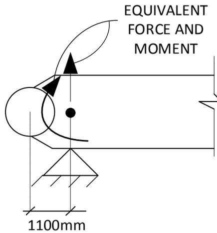
**FIGURE 61: EQUIVALENT FORCE AND MOMENT DUE TO ECCENTRICITY OF FRONT TRUNNIONS**
