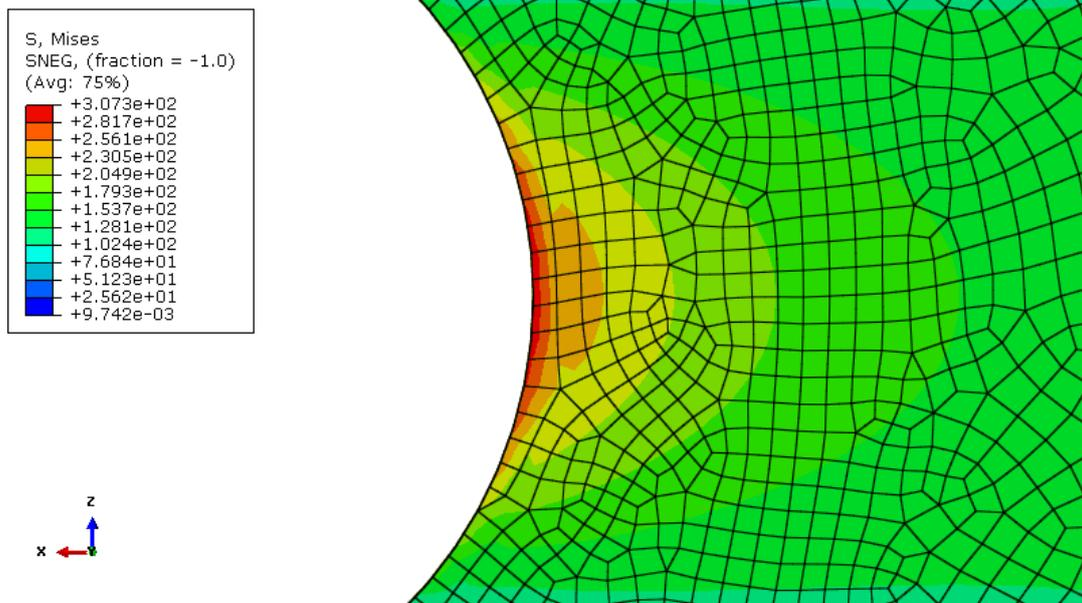
FIGURE 93: STRESS CONCENTRATION OF FRONT TRUNNION
