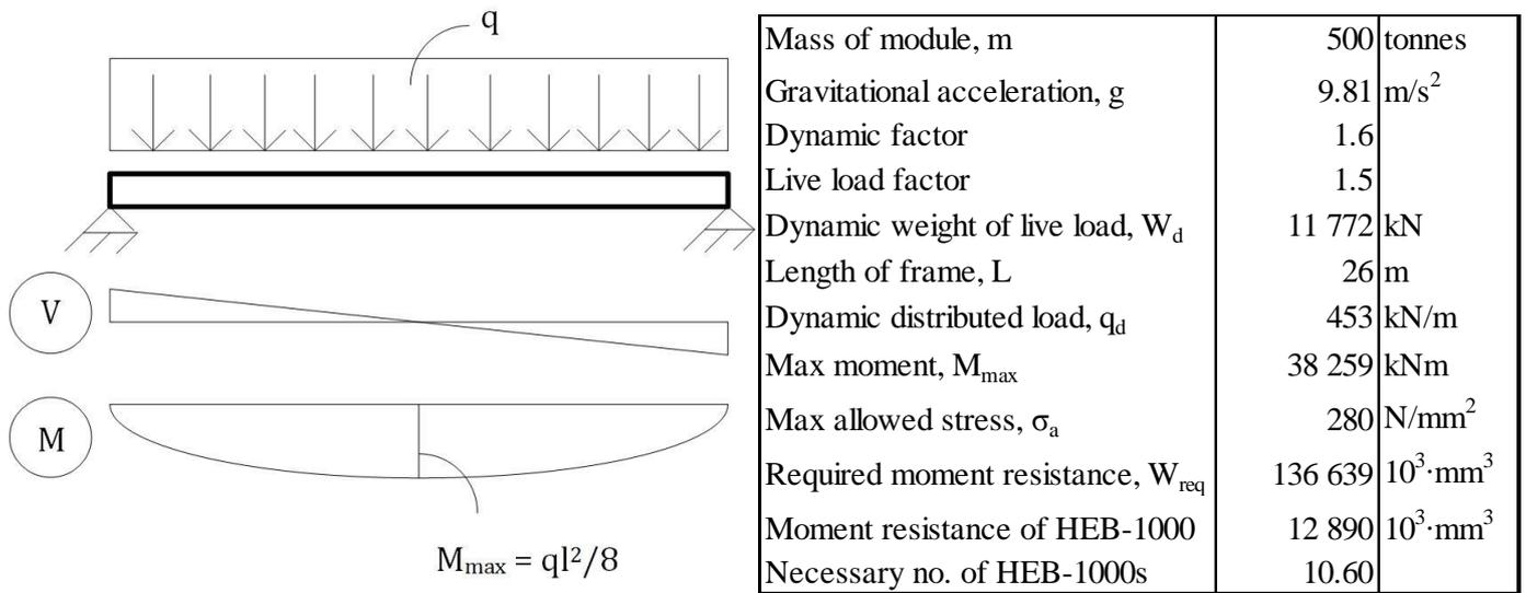
FIGURE 12: SIMPLE CALCULATION OF MOMENT RESISTANCE
