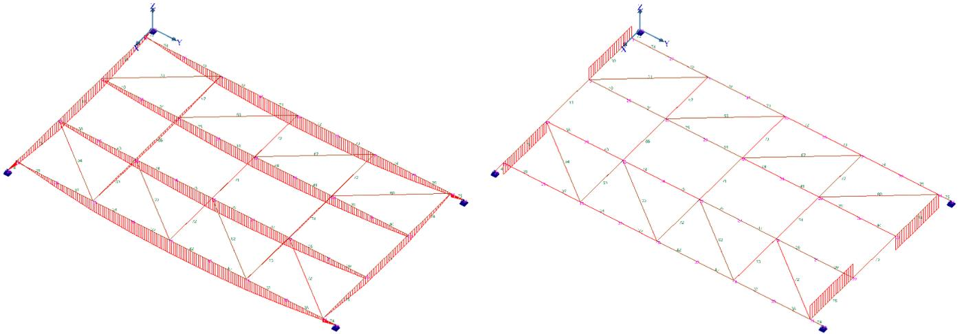
FIGURE 98: MOMENT AND TORSION DIAGRAM, HORIZONTAL POSITION
