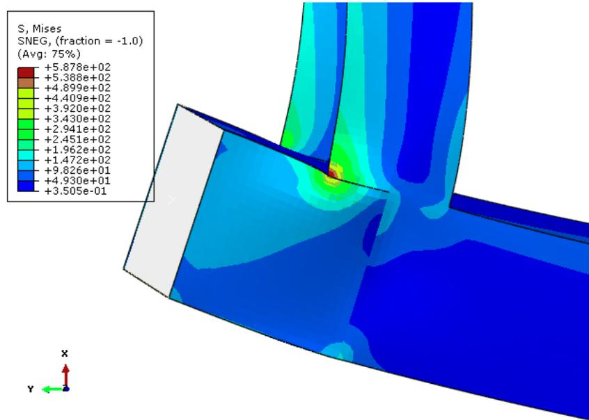
FIGURE 89: STRESS CONCENTRATION IN VERTICAL POSITION
