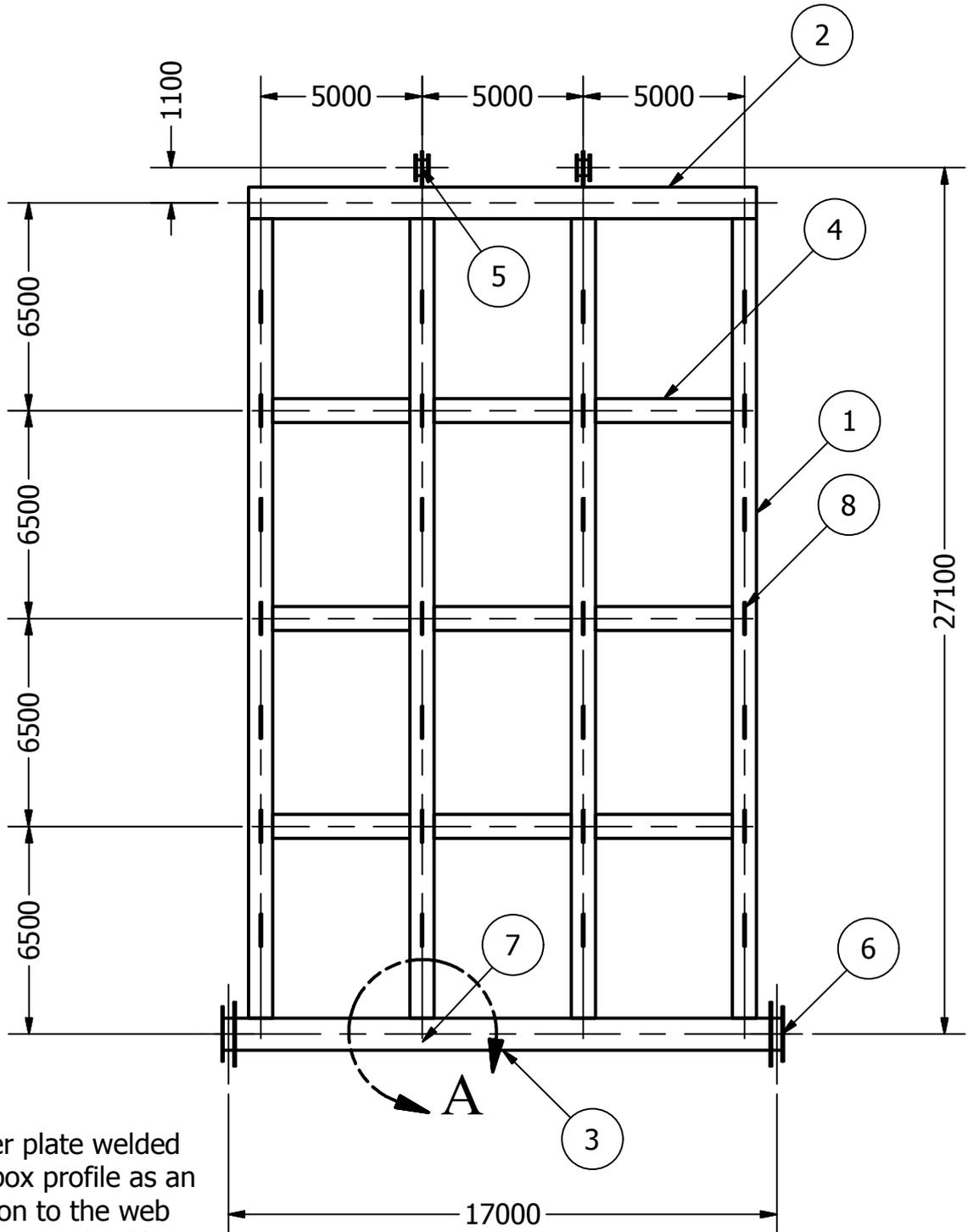
Stiffener plate welded inside box profile as an extension to the web of the longitudinal beam
