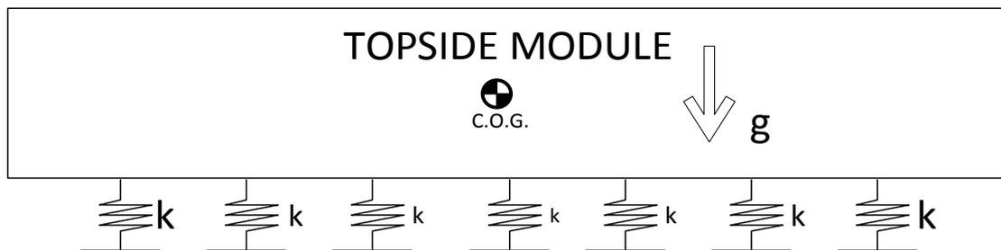
**FIGURE 38: SPRING-LIKE SUPPORT OF THE TOPSIDE MODULE**
