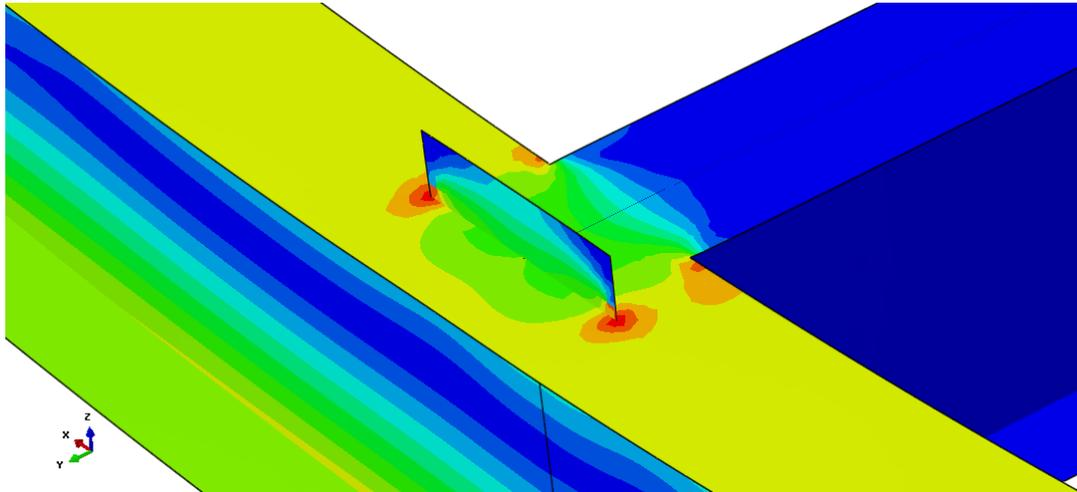
FIGURE 87: STRESS SINGULARITIES OF SHEAR PLATES
