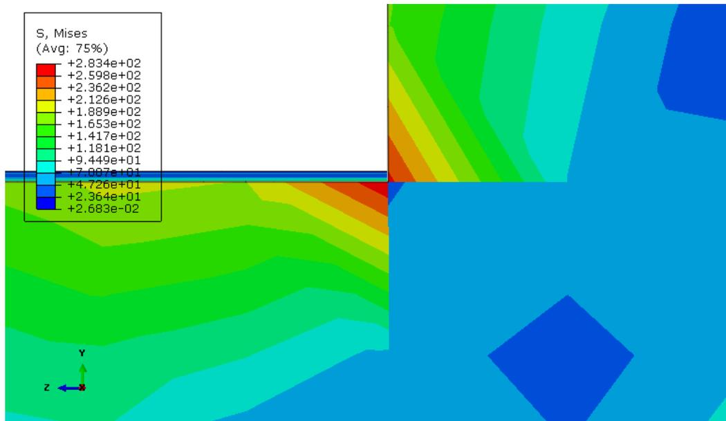
FIGURE 96: ILLUSTRATION OF THE DEPTH OF THE CRITICAL STRESS AREA IN HORIZONTAL POSITION
