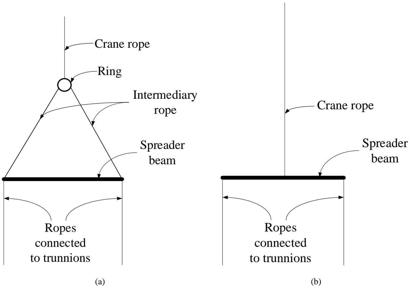
FIGURE 30: SUGGESTIONS TO ARRANGEMENT OF LIFTING EQUIPMENT
