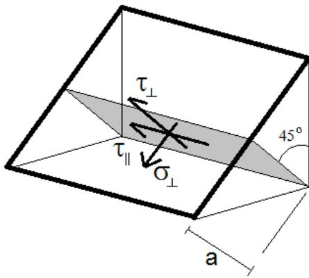
FIGURE 68: CROSS SECTION OF WELD WITH INTERNAL FORCES
