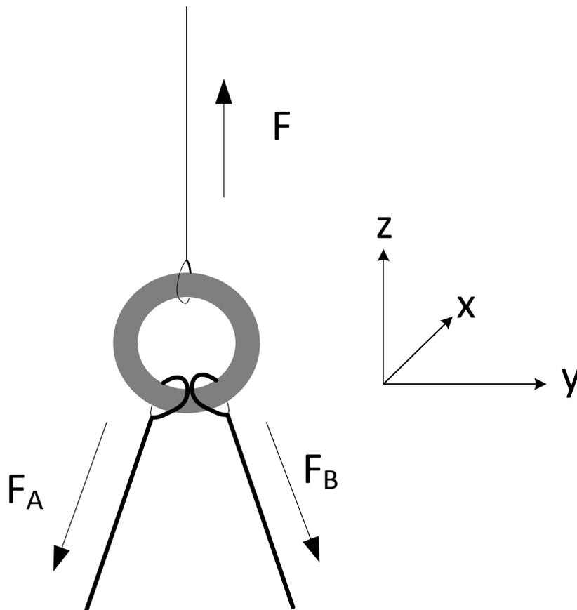
FIGURE 51: RING JOINT CONNECTING ROPES
