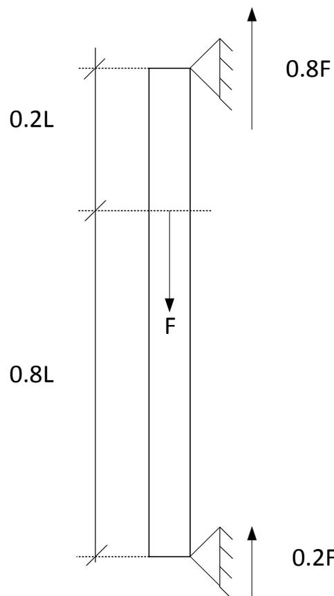
FIGURE 64: CONSTANT AXIAL STIFFNESS ASSUMPTION OF FRAME
