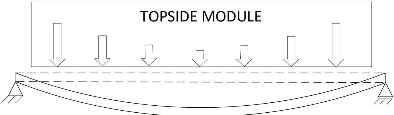
FIGURE 39: LOAD TRANSFER BETWEEN MODULE AND FRAME GIVEN THAT THE MODULE IS STIFFER
