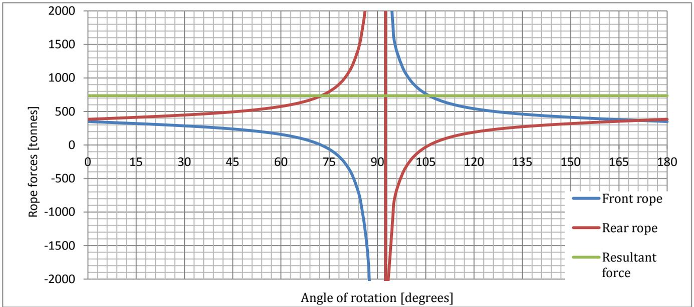
**FIGURE 53: ROPE FORCES NECESSARY TO MAINTAIN EQUILIBRIUM WITH VERTICAL ROPES**
