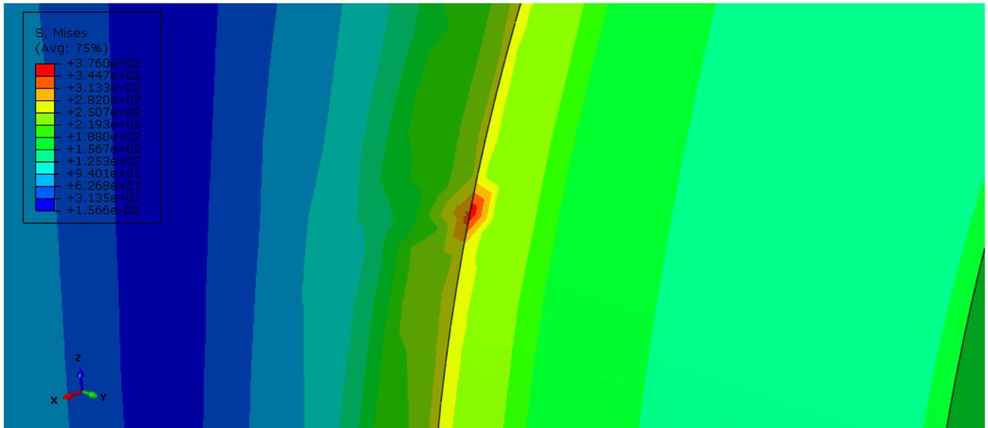
**FIGURE 97: PEAK STRESS IN REAR TRUNNION IN VERTICAL POSITION**
