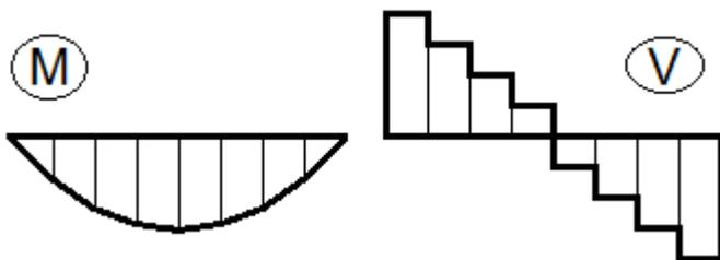
FIGURE 70: APPROXIMATE MOMENT AND SHEAR FORCE DIAGRAM FOR THE LOADED FRAME
