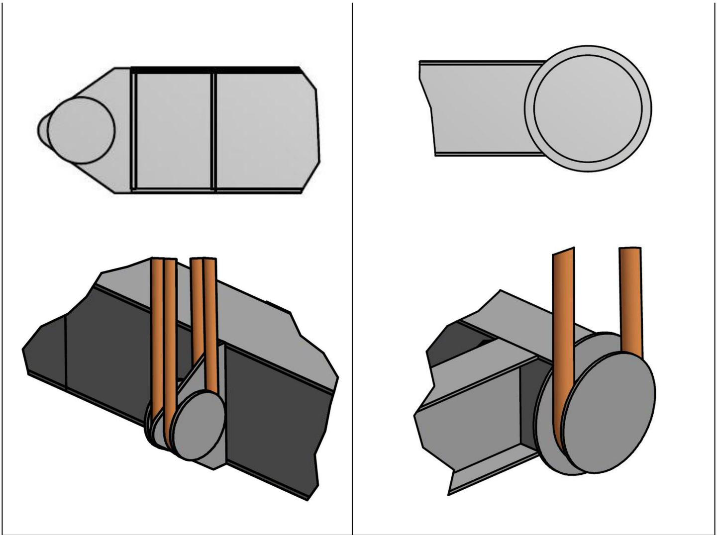
From the illustration of the front trunnion, it is visible that the ropes are eccentric from the center of the front beam. This eccentricity is 1100mm. The trunnion in the rear is eccentric 1000mm from the centerline of the nearby longitudinal, but coincides with the centerline of the rear beam.
