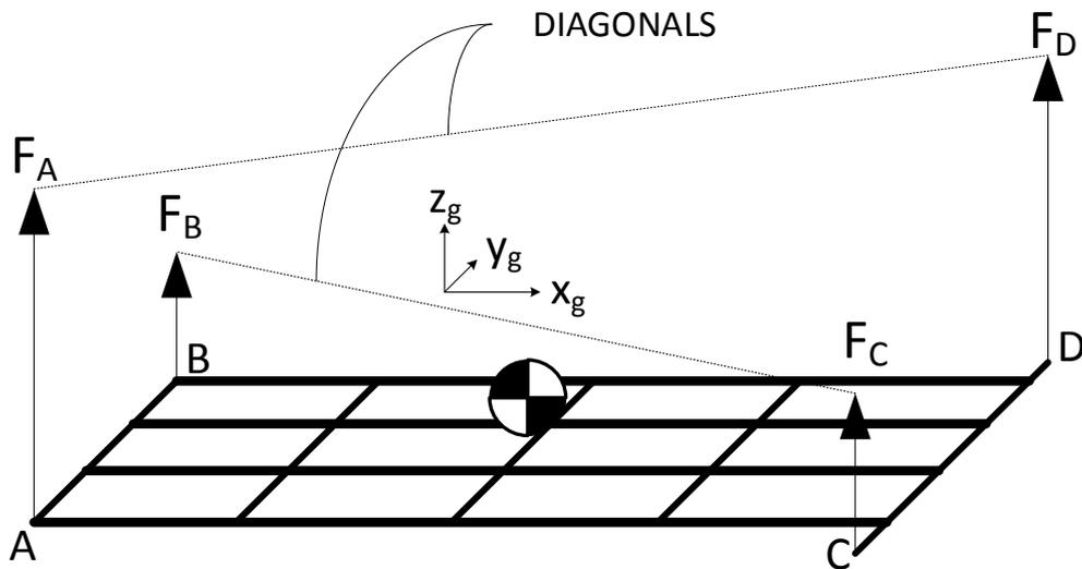
FIGURE 50: SKEW LOAD FACTOR DUE TO STATIC INDETERMINACY
