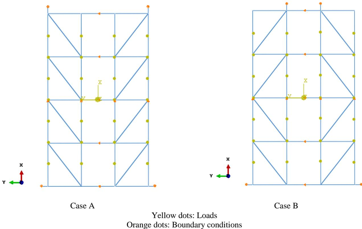
**FIGURE 75: LOADS AND BOUNDARY CONDITIONS IN HORIZONTAL POSITION**
