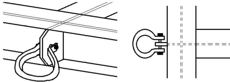
FIGURE 15: LIFTING LUG WITH SHACKLE
