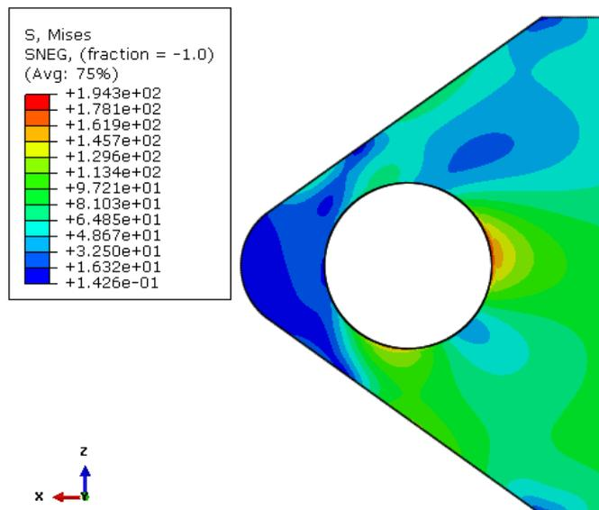
FIGURE 92: STRESS AND DEFORMATION OF FRONT TRUNNION IN 2)b) VERTICAL POSITION
