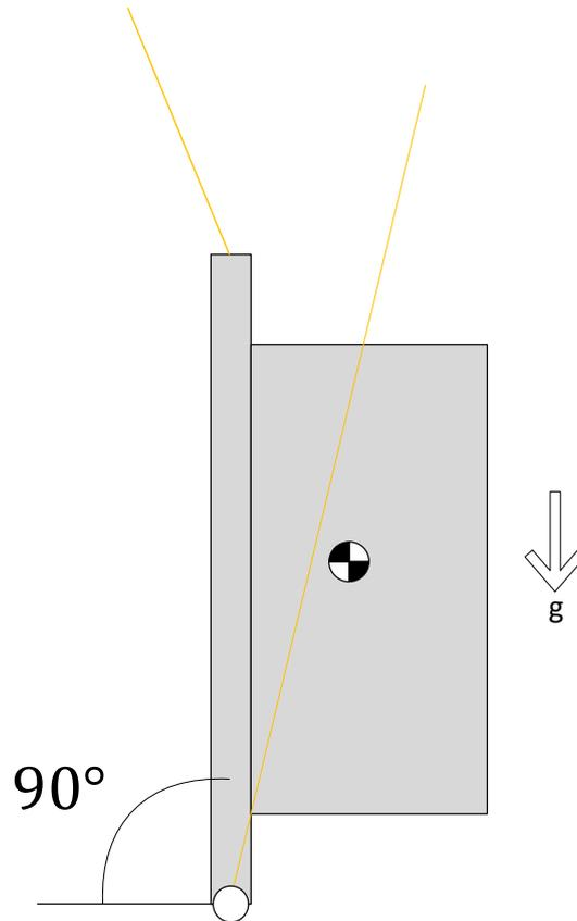
FIGURE 52: INSTABILITY IN VERTICAL POSITION
