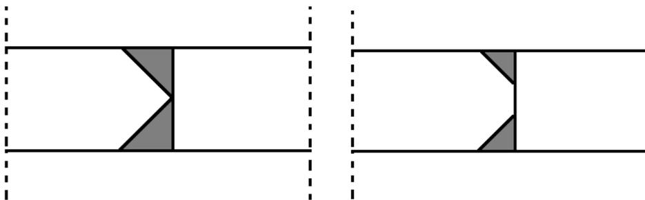
FIGURE 66: BUTT WELD WITH/WITHOUT FULL PENETRATION
