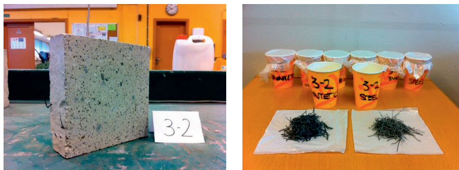
Fig. 3.8. Polymer and steel fibres contained in a slice of standard beam.
