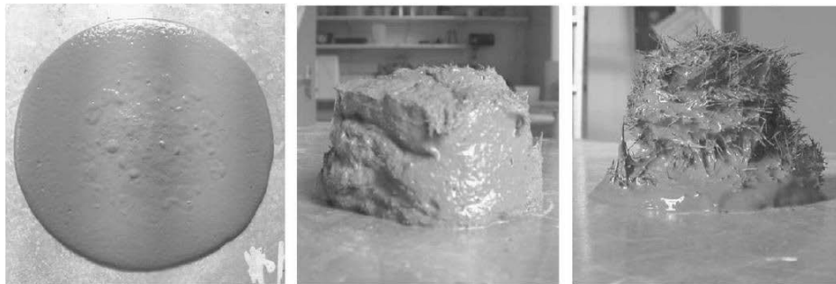
Fig. 2.1. Effect of increasing the fibre factor ( v_f \cdot l_f/d_f ) on the consistency of a cement paste mixed with fibres (Martinie et al., 2010).
