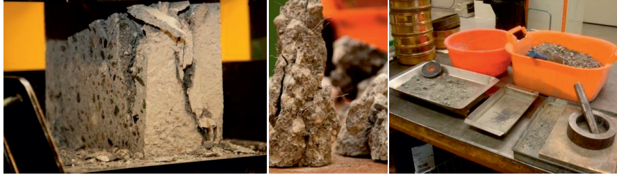
Fig. 2.7. Determination of the fibre content in a hardened concrete sample (Sarmiento, 2011).
