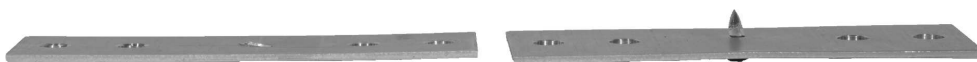
Figure 4.24: Screwed C-90 test specimen after deformation. The upper side of the bottom sheet is seen to the left and the underside of the top sheet is seen to the right.
