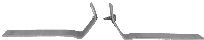
Figure 4.29: Screwed P test specimen after deformation. Top sheet is to the right.
