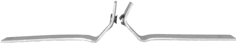
Figure 4.17: Riveted P specimen after deformation. Top sheet is to the right.
