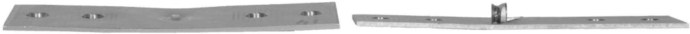
Figure 4.11: Riveted C-90 test specimen after deformation. The upper side of the bottom sheet is seen to the left and the underside of the top sheet is seen to the right.
