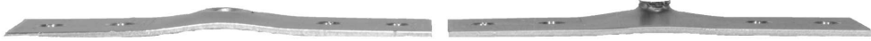
Figure 4.9: Riveted C-45 test specimen after deformation. The upper side of the bottom sheet is seen to the left and the underside of the top sheet is seen to the right.
