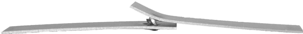
Figure 4.14: Riveted SLJ test specimen after deformation. Top sheet is to the right.
