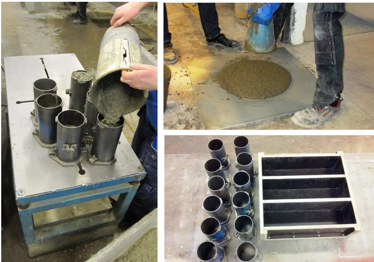
Figure 4.4. Left: Casting of test cylinders on a vibrating table. Upper right: Slump test. Lower right: Formwork for the fibre test beams and cylinders.
