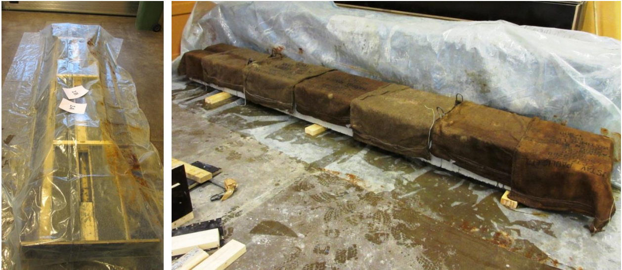
Figure 4.5. Left: Beams covered in plastic directly after casting. Right: Beams covered in burlap sacks after removal from the formwork and then covered in plastic again.
