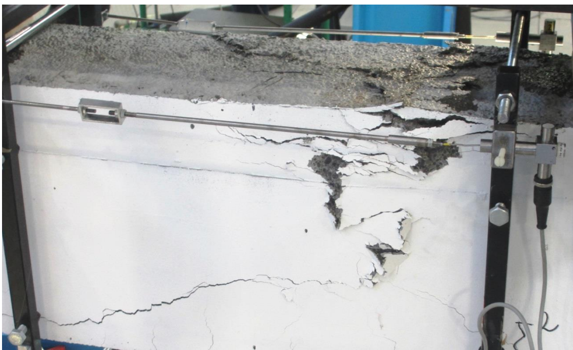
Figure 6.24. Final cracking on the top and west side of beam 2B.
