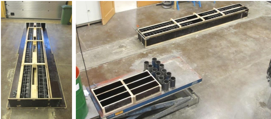
Figure 4.3. Overview of the laboratory with formwork for beams and test specimens ready for casting.
