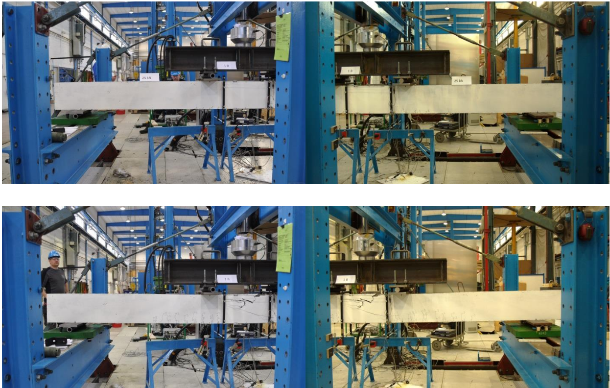
Figure 5.4. Example of the loading procedure for beam 1B from two angles. 25 kN load in the upper pictures and cracking at end of test in the lower picture.
