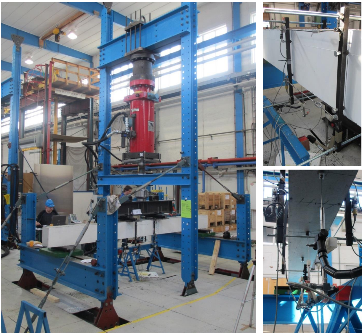
Figure 5.1. Left: Testing rig in the laboratory with the beams north end on the left side on the picture and the south end on the right side of the picture. Upper right: Strain sensors on the beams west side. Lower right: Deflection sensors on the underside of the beam.
