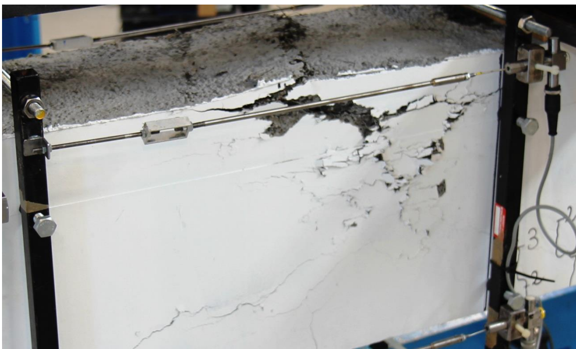
Figure 6.31. Final cracking on the top and west side of beam 3B.
