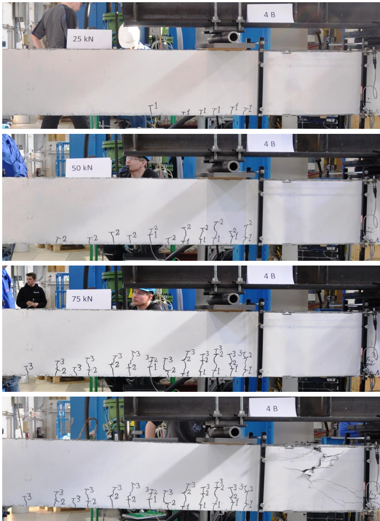
Figure 5.5. Test procedure for beam 4B. The load at each loading level is indicated on the pictures but the last picture shows the cracking at mid span for the final load at the end of test.
