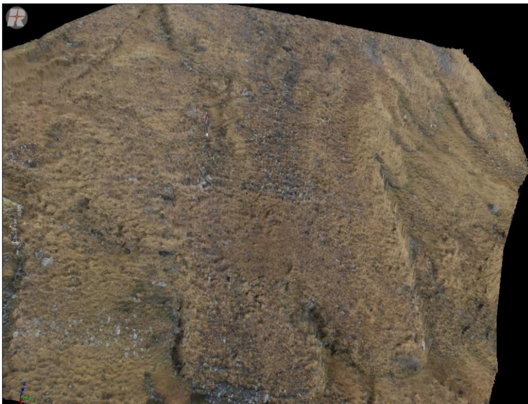
Figure 5.5. DEM of solifluction lobe from 2014, textured with photos from the scan campaign, smoothed and decimated
