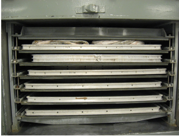
Figure 18.2: The aluminum tray with the fish blocks in between the plate thawer walls
