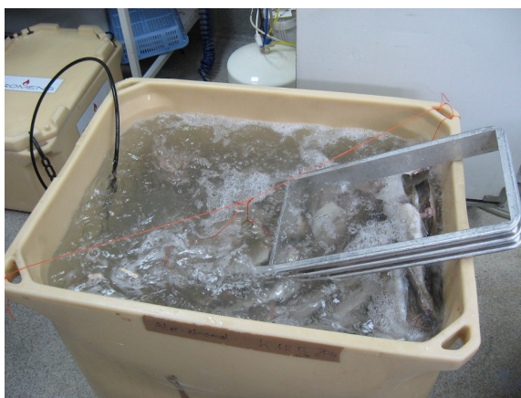
Figure 4.2: Thawing of two blocks of frozen H/G cod in a tank with enhanced heat transfer due to air bubbles - the aluminum frame hinders the fish blocks from being lifted up
