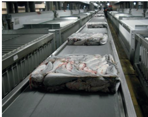
Figure 3.2: Fish blocks on a conveyor belt after having been frozen in vertical plate freezers (left and right from the conveyor belt) on board a fishing vessel
