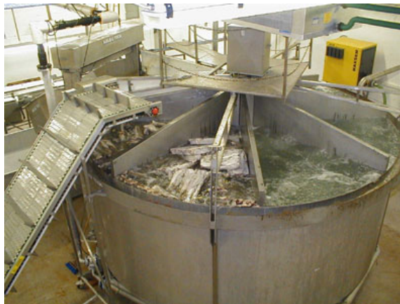
Figure 4.3: A cylindrical thawing tank as built by Melbu Systems AS, Melbu, Norway
