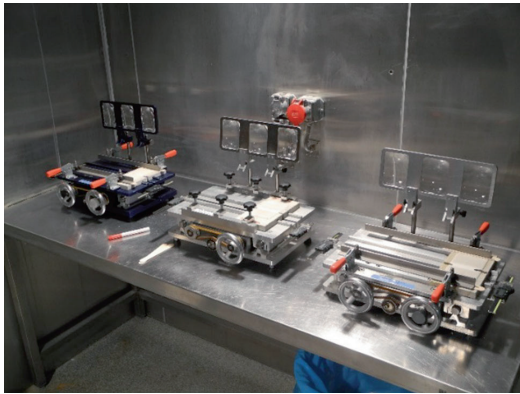
Fig. 14 Crack bridging testing with adopted procedure in progress in climate chamber. (Courtesy by Wacker Chemie AG)
