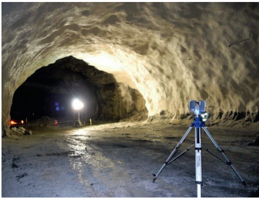
Fig.11 Interior of the Karmsund test site with the waterproofing membrane recently applied, and LiDar scanning of the surface in progress.
