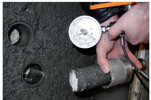
Fig. 16 Adopted procedure for in situ measurements of tensile bonding strength. Top conceptual diagram showing the layout of the test. Middle Preparation with over-coring with grinding of the test specimen. Bottom in situ specimen after testing
