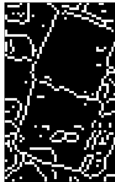
(d) Edge detection of (a) by the derivative using Sobel edge detector with the threshold of 0.01. More weak edges (non-closed) between the connected floes are found at the cost of more noise.
