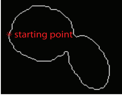
Figure 4.5: A boundary's chain code and its first difference.
