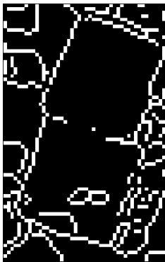
(c) Edge detection of (a) by the derivative using Sobel edge detector with the threshold of 0.02. Part of the weak edges (non-closed) between the connected floes are found.
