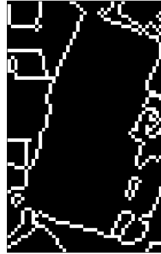
(b) Edge detection of (a) by the morphology method. The detected boundaries are closed, but the weak edges between the connected floes are lost.
