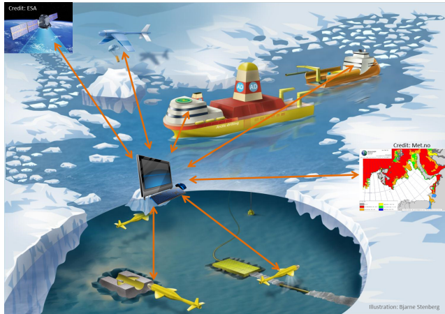
Figure 1.5: Ice intelligence system collects and analyzes the ice environment information from surface and subsurface scouting tools. Illustration by Bjarne Stenberg. Copyright: NTNU
