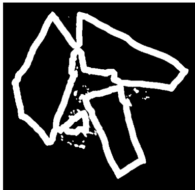
(c) Edge detection of (a) by the morphology method using the internal gradient with a 16-pixel-radius disk-structuring element. The detected floe boundaries become thicker, and the weakly connected ice floes are separated.
