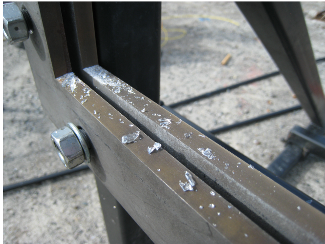
Figure 46: Glass pieces on frame after explosion on thin plate with 75 cm stand-off.
