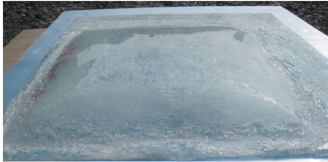
Figure 45: Permanent deformation of laminated pane, 75 cm stand-off on thick plate.
