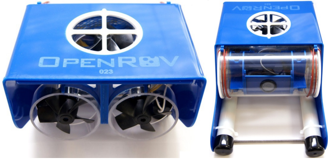
Fig. 1. OpenROV, an open source underwater robot for educational purposes.
