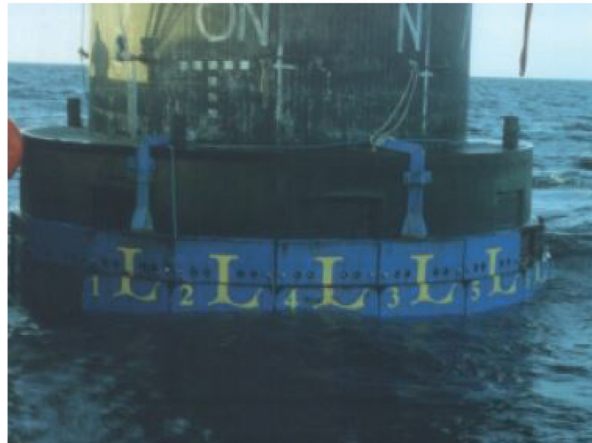
Figure 5. The Nordströmsgrund lighthouse: a) picture of the concrete structure in ice-infested water; b) force panels mounted to the outer face.
