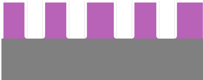
Figure 3.9: The desired profile of the pattern of holes after HF wet etching. In this figure the etching time is just right. The etching has just etched through the entire initial width of the holes, but no excess widening has occurred.
