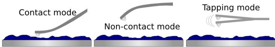
Figure 2.29: Illustration of the different operation modes of the AFM. To the left the contact mode can be seen in operation, where the tip is in contact with the substrate during the measuring. In the middle the non-contact mode can be seen in operation, where the tip hovers above the substrate to measure interaction forces during measuring. The the right the tapping mode can be seen in operation, where the tip taps up and down to lessen damage and avoid sticking to the surface.
