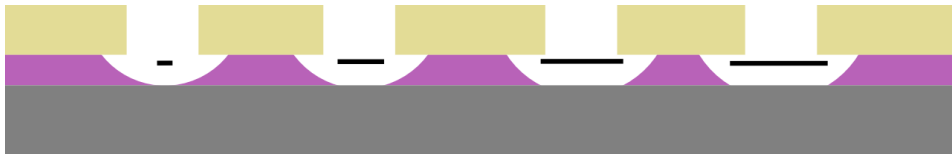
Figure 4.1: Illustration of the HF etch profile of a previously tried out etching technique. Here the problems with HF wet etching directly on the PMMA covered \text{SiO}_2 layer on \text{Si}(111) are illustrated. As seen in the illustration, the etch profile gets very isotropic as the HF seems to get in between the PMMA and \text{SiO}_2 interface during the etching. This results in very uncontrolled hole sizes on the \text{SiO}_2 and \text{Si}(111) interface. A small difference in etch rate can result in large differences in the \text{SiO}_2 - \text{Si}(111) interface holes, as illustrated by the black lines. The black lines demonstrate the length of the diameter of the \text{SiO}_2 - \text{Si}(111) interface of the different holes.
