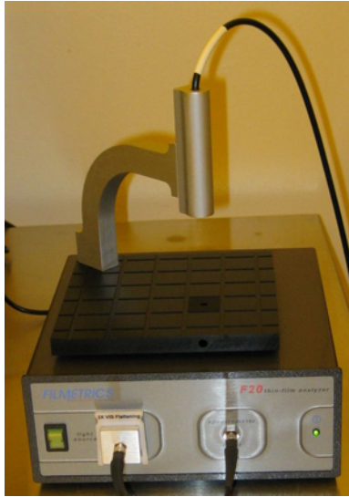
Figure 3.3: One of NTNU NanoLab’s reflectometers. This instrument can be found in the second innermost lithography and wet etch lab finger. This is an F20 model by Filmetrics.
