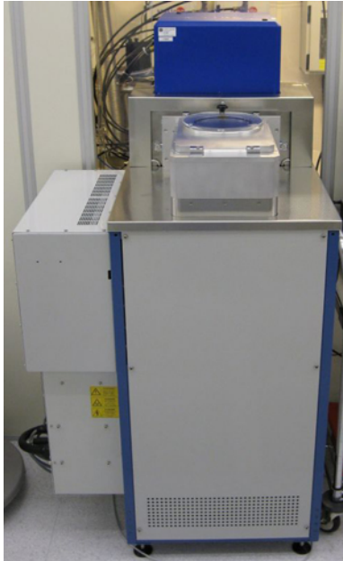
Figure 2.2: NTNU NanoLab's PECVD system. This instrument can be found in the innermost thin film and dry etch lab finger.
