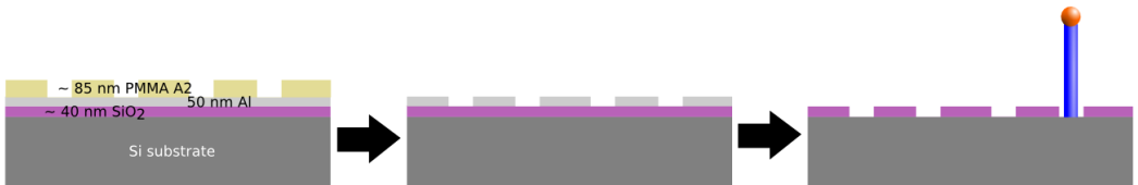
Figure 3.2: Illustration of the overall experimental procedures of this master's thesis. During various procedures and various layers of material, including, Si, SiO 2 , Al and PMMA, the goal is to obtain an ordered array of nanoscaled holes of ~ 100 nm, made by anisotropic dry etching on a Si(111) substrate, for growth of nanowires.
