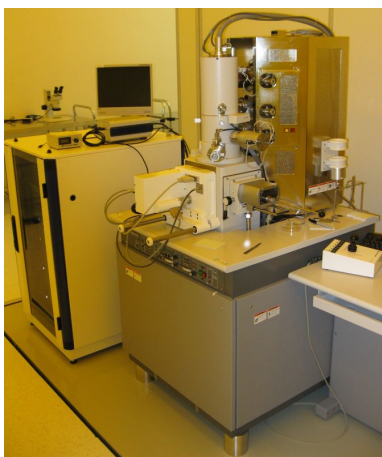
Figure 3.6: NTNU NanoLab's EBL system. This is a Hitachi 4300 SEM with Raith laser stage model. This instrument can be found in the second innermost lithography and wet etch lab finger.
