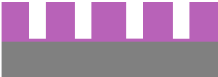
Figure 3.8: Illustration of a thin \text{SiO}_2 layer at the bottom of the patterned holes. After the dry etching, the patterned holes are likely to have a thin \text{SiO}_2 layer at the bottom, covering the Si(111) substrate. This layer is important to remove in order to have NW growth on the underlying silicon.
