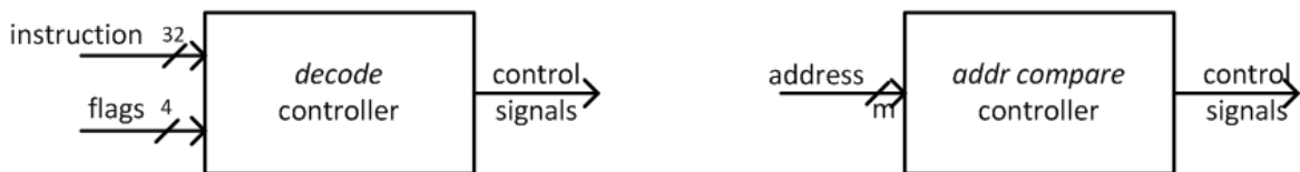
Figure 3.7 – Two different Loop Cache Controller implementations and their interfaces
