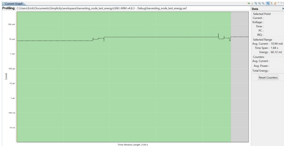
Figure 4.1: Energy trace of node's initialization.
