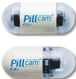
Figure 1.1: Two PillCam models from Given Imaging. The upper capsule is designed for inspection of the esophagus, while the one at the bottom is for use in the small intestine. Picture from [3], used with permission.
