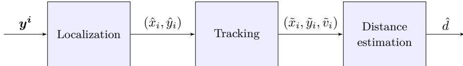
Figure 3.1: Overview of the localization and tracking system.
