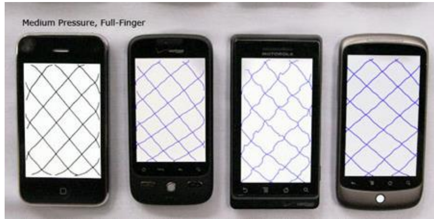
Figure 3.3: Comparison of signal processing capabilities on mutual capacitance touch screens 5
