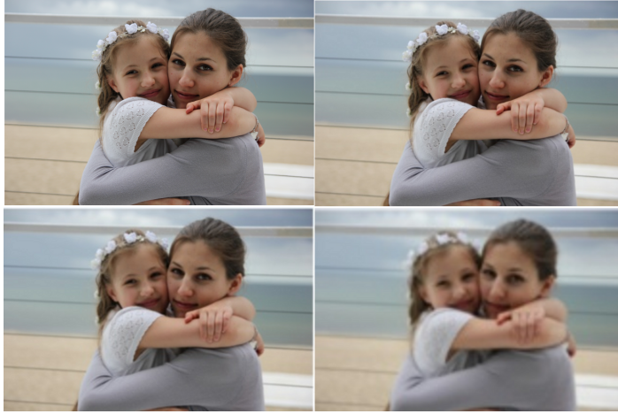
Figure 3.6. Laplacian Pyramid with four levels, first row from the left level 0, 1, second row level 2, 3
