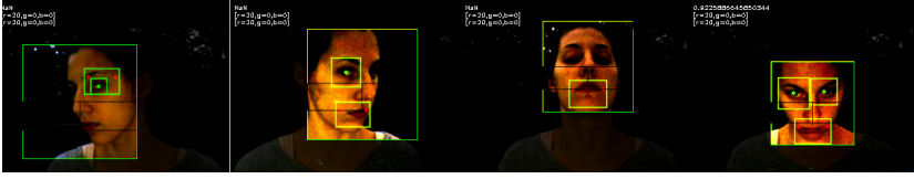
Figure 6.7. A picture taken for different head positions, from left: + 45 horizontal, -45 horizontal, +30 vertical, -30 vertical
