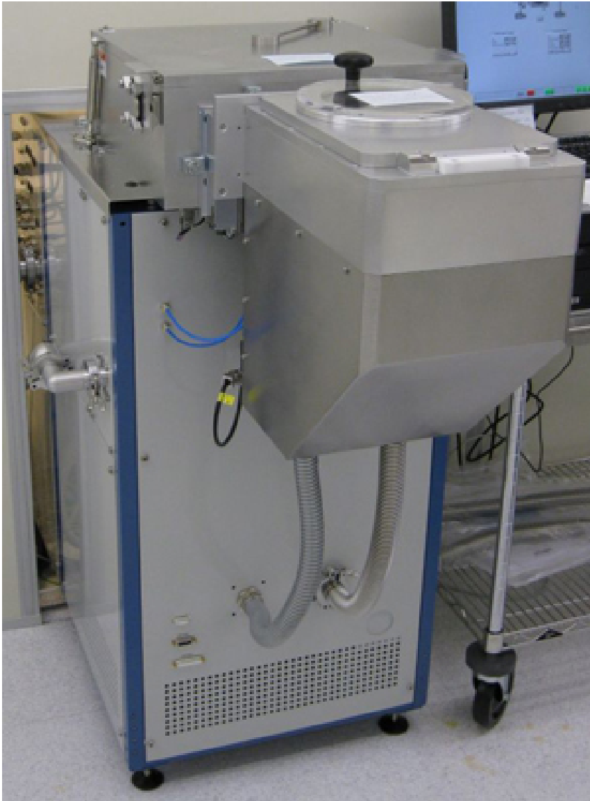
Figure 3.7: The Oxford Instruments Plasmalab System 100 ICP-RIE 180 installed at NTNU NanoLab.
