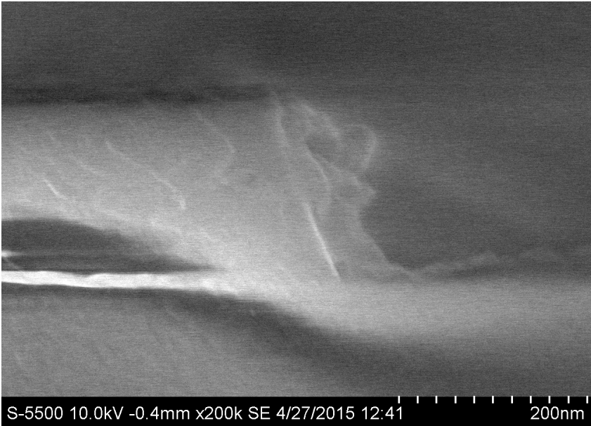
Figure 4.21: Cross-section image of slightly tapered sidewalls etched in amorphous SOI with Recipe 18 at a dose of 180 \mu\text{C}/\text{cm}^2 and with 270 nm thick resist.
