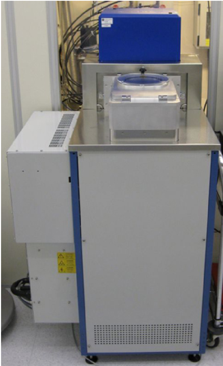
Figure 3.10: The Oxford Instruments Plasmalab System 100 PECVD installed at NTNU NanoLab.
