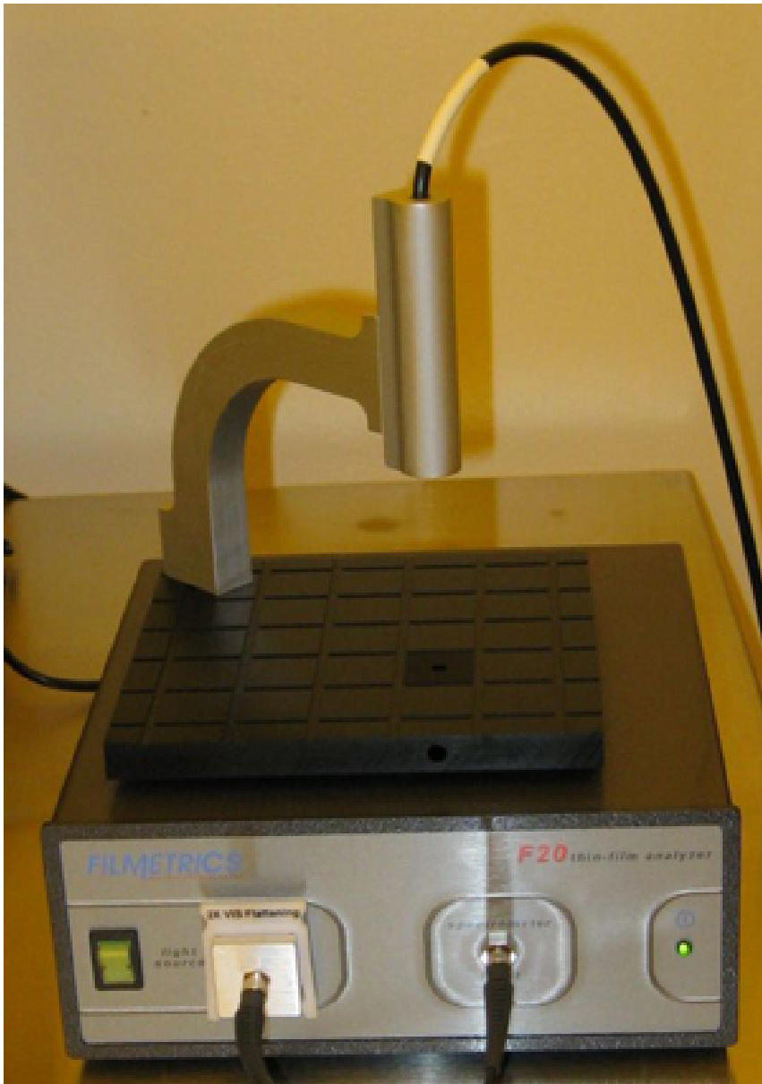
Figure 3.11: The Filmetrics F20 reflectometer installed at NTNU NanoLab.
