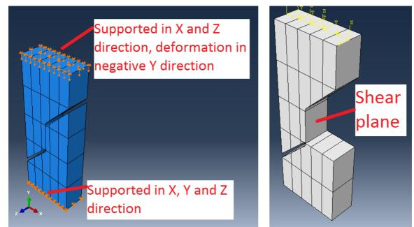
Figure 7: Support and load application
