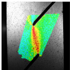
Figure 29: Typical contour plot of shear strains from ARAMIS
