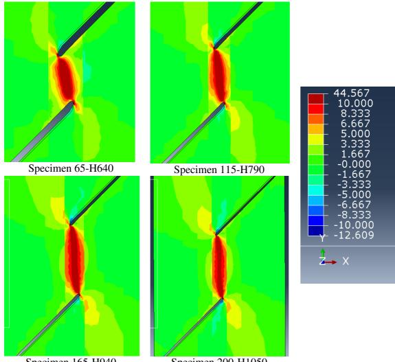
Specimen 165-H940Specimen 200-H1050Figure 42: Contour plots of surface shear stress for specimens modelled in part three
