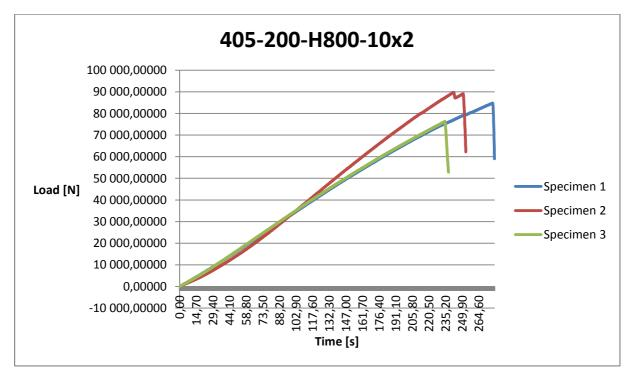
Figure 53: Load (N) versus time (s) plotted for specimen 405-200-H800-10x2 from part two
