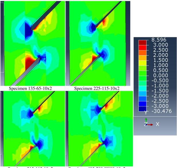
Specimen 315-165-10x2Specimen 405-200-H800-10x2Figure 25: Contour plots of normal stress perpendicular to fibres for specimens in part two
