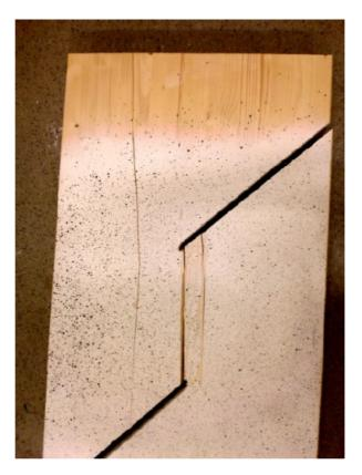
Figure 38: Cracks forming from top of specimen
