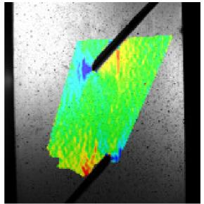
Figure 30: Typical contour plot of normal strains perpendicular to fibres from ARAMIS
