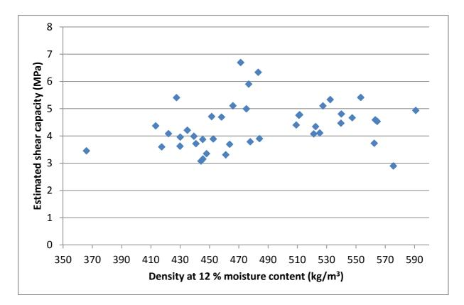
Figure 44: Estimated shear strength plotted against density
