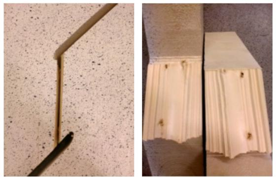
Figure 26: Specimen split in half at failure forming one shear plane
