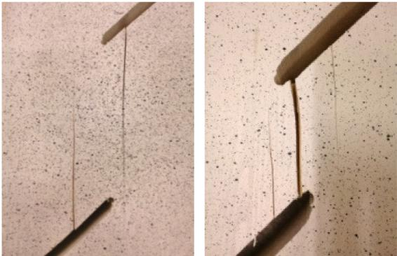
Figure 27: Two cracks formed at failure
