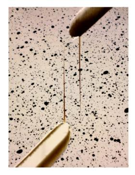
Figure 20: Two vertical cracks forming between cuts
