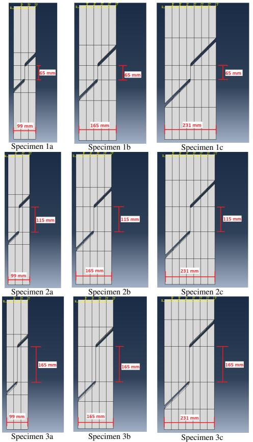
Figure 12: The nine first specimens modelled in ABAQUS. All specimens have a total height of 600 mm and are 90 mm deep. The height of the shear plane and the width of the specimens vary as shown above.
