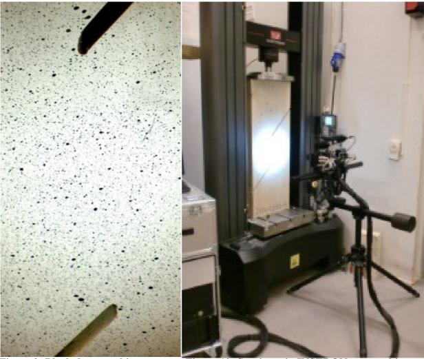
Figure 9: Black dots on white background for video extensometry
