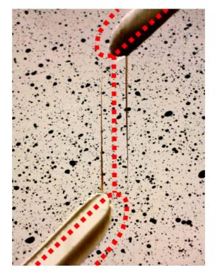
Figure 21: The red dashed line illustrates how the cuts should be moved deeper into the specimen in order to form one shear plane instead of two cracks
