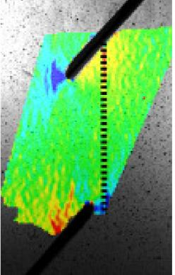
Figure 34: Path used for plotting of normal strains perpendicular to fibres
