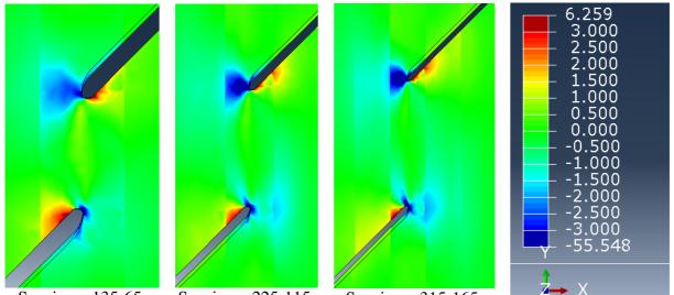
Specimen 135-65 Specimen 225-115 Specimen 315-165 Figure 19: Contour plots of surface normal stress  $\sigma_X$  for glulam of 45 mm lamina used for laboratory testing in part one
