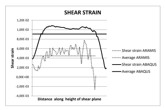
Figure 35: Shear strain from ARAMIS (dotted) and ABAQUS (solid) plotted against the height of the shear plane
