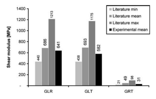
Figure 5: Shear moduli found by Dahl and Malo (2009a) compared to literature min, literature mean and literature max (Dahl & Malo, 2009a)
