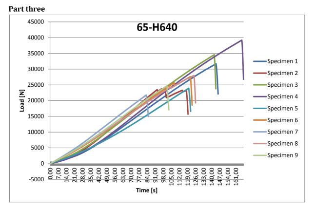
Figure 54: Load (N) versus time (s) plotted for specimen 65-H640 from part three
