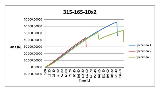
Figure 52: Load (N) versus time (s) plotted for specimen 315-165-10x2 from part two
