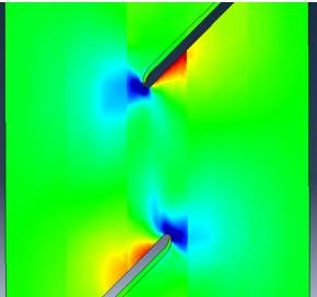
Figure 32: Typical contour plot of normal strains perpendicular to fibres from ABAQUS
