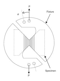
Figure 4: The Arcan shear test
