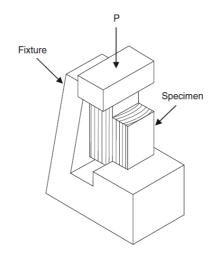
Figure 1: Notched shear block test
