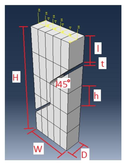
Figure 6: Specimen used for investigation of shear properties: H is the total height, W is the width, D is the depth, h is the height of the shear plane, t is the thickness of the cut and I is the length of wood continuing above (or below) the cut.
