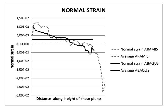
Figure 36: Normal strain perpendicular to fibres from ARAMIS (dotted) and ABAQUS (solid) plotted against the height of the shear plane
