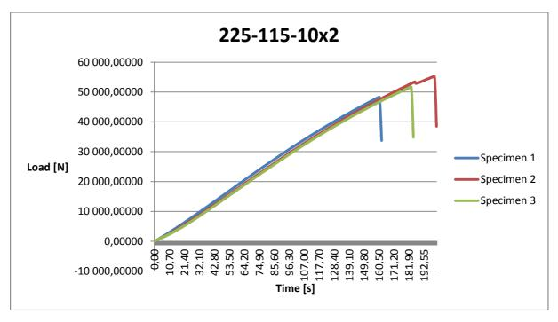
Figure 51: Load (N) versus time (s) plotted for specimen 225-115-10x2 from part two
