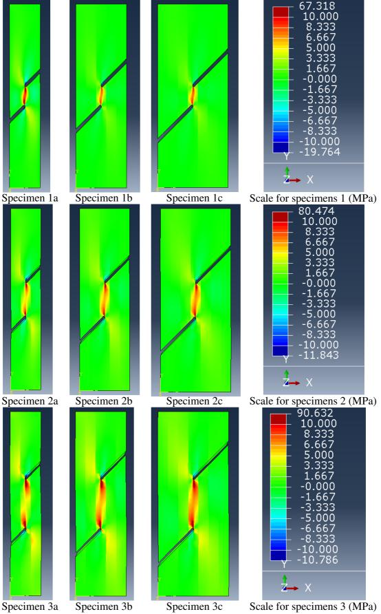
Figure 17: Contour plots of surface shear  $\tau_{XY}$  for glulam of 33 mm lamina
