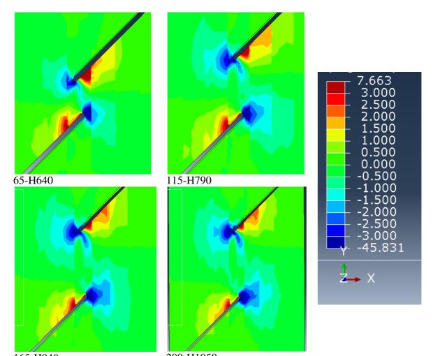
165-H940200-H1050Figure 43: Contour plots of surface normal stress perpendicular to fibres for specimensmodelled in part three
