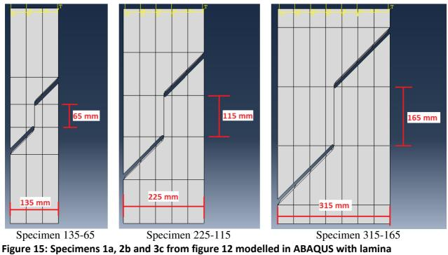
thickness 45 mm to be tested in the lab.
