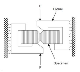
Figure 3: The losipescu shear test
