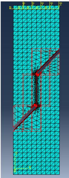
Figure 13: A fine mesh is applied around the ends of Figure 14: The red boxes show the cuts and along the shear plane.
