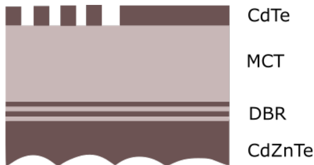
Figure 3.1: Illustration of a cross section of the structure used in the PL spectroscopy experiments. The thickness and width of the different layers are not to scale.
