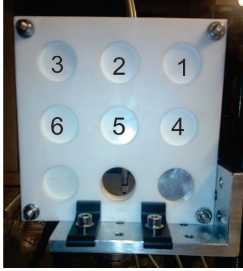
Figure 6.3: Sample holder with samples, numbered from 1-6, according to Table 6.2.
