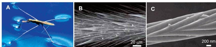
**Figure 3.18:** (a) A pond skater resting on water. (b) SEM image of a pond skater leg covered with micro-sized hairs. (c) SEM image of nanogrooved structure on the hairs.<sup>[38]</sup>
