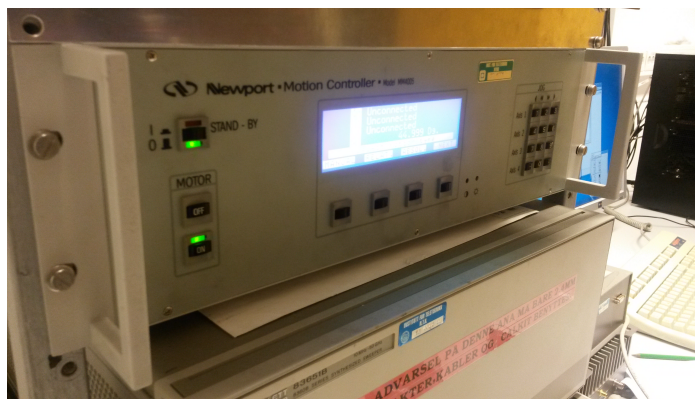
Figure 6.4: Motion controller rotating the platform with the receiver antennas.
