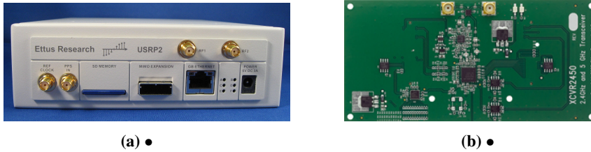
Figure 5.1: a) Ettus Research USRP2. b) RF Daughter Board XCVR2450 in the USRP2.
