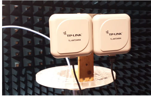
Figure 4.3: The 9 dBi tracking antennas used for DOA estimation.
