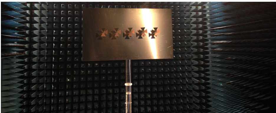
Figure 5.1: The 5-element crossed bowtie array mounted in the anechoic chamber at NTNU
