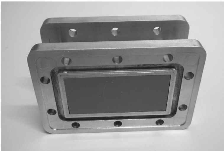
Figure 5.4: Radome sandwich sample inserted in sample holder.
