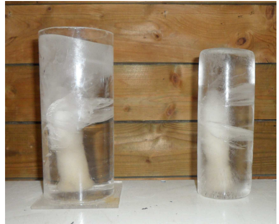
Figure 29 - Ice cylinders with and without formwork
