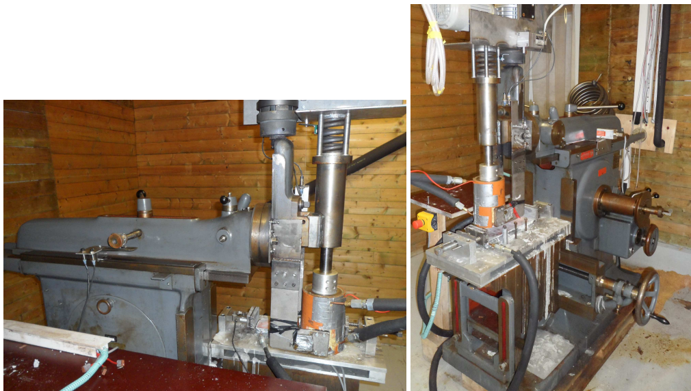
Figure 21 - NTNU Ice abrasion apparatus, the grey metal plane machine
