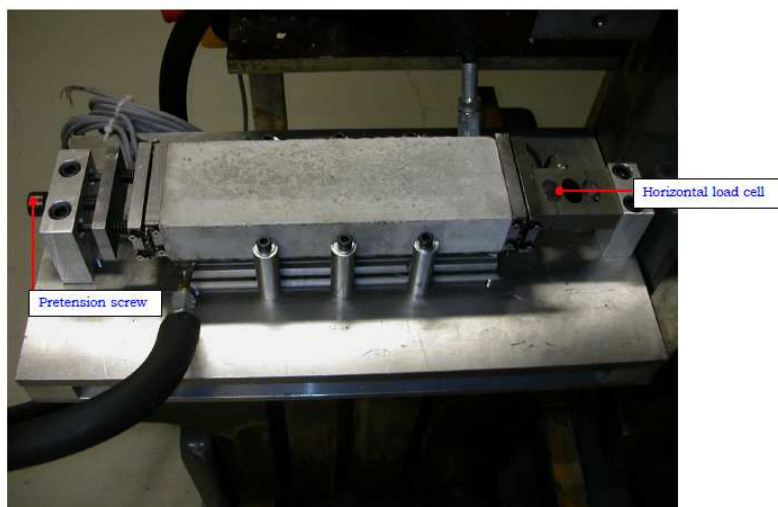
Figure 23 - NTNU Ice abrasion apparatus, concrete bedding
