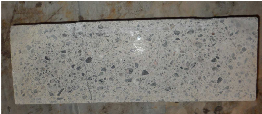
Figure 34 - Picture of concrete sample B1 after abrasion testing
