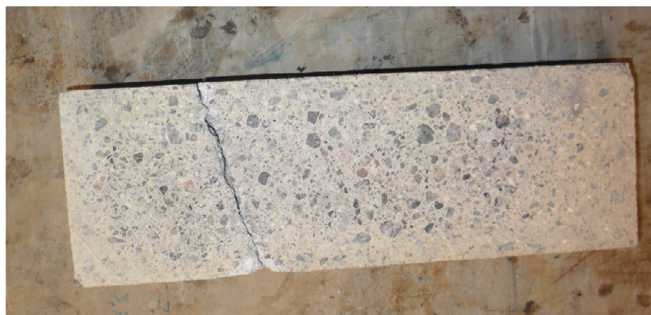
Figure 36 - Picture of concrete sample A2 after abrasion testing
