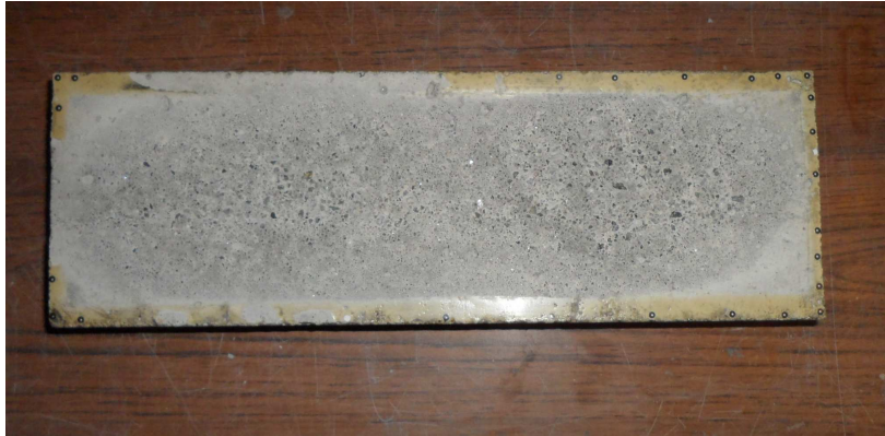
Figure 25 - Concrete sample with self-adhesive circular marks
