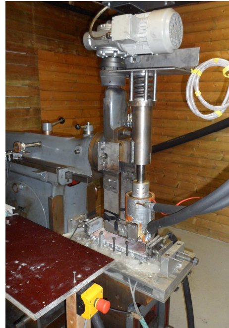
Figure 22 - NTNU Ice abrasion apparatus, insulated cylinder and vertical pressure engine
