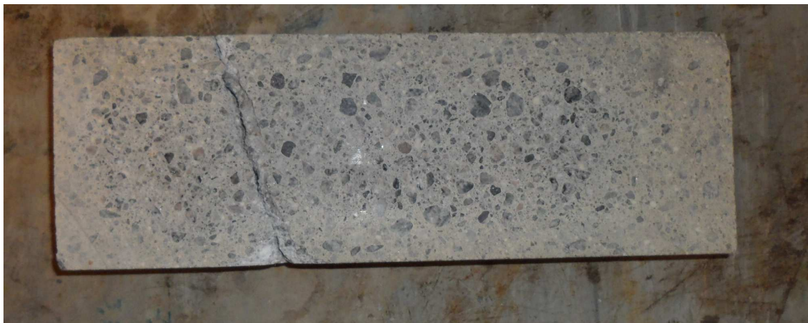
Figure 38 - Picture of concrete sample B2 after abrasion testing
