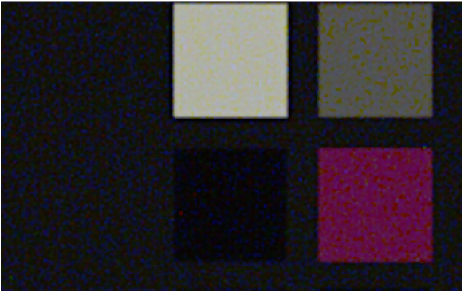
Figure 5.12: Top left part of test scenario 1, when it has been filtered with the proposed algorithm, modified Yaroslavsky N_{4,5} . The noise have been blurred, but edges are kept sharp. Note that the red impulse in the black square has been emphasized, because the impulse originally spans over several pixels.
