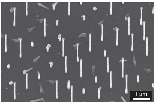
Figure S7. Tilted-view SEM image of GaAs NWs grown without an annealing step prior to the NW growth, showing a substantial reduction in the yield. Apart from the substrate annealing treatment, all other growth conditions were the same that result in a yield of \sim 80\% , i.e. Ga predeposition time of 50 s, Ga rate of 0.6 \text{ MLs}^{-1} and \text{As}_2 flux of 5.0 \times 10^{-6} \text{ Torr} for at a growth temperature of 630 \text{ }^\circ\text{C} .
