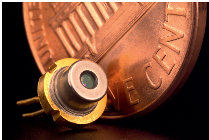
Figure 1.2: A photograph of a packaged laser diode, showing its small size. The actual laser diode is usually only a few mm long, and it is placed behind the window of the laser package. This photograph is downloaded from Wikimedia Commons [5].
