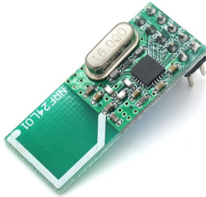
Figure 2.2: nRF24L01 (one of its variants), a purely embedded solution
