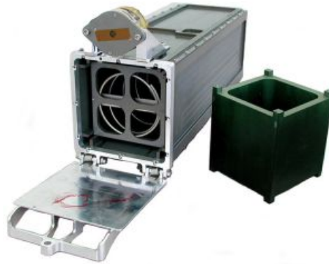
Figure 1.2: P-POD launch mechanism and mock 1U CubeSat
