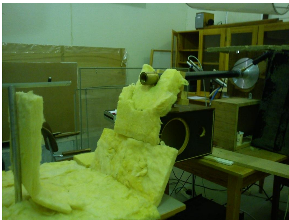
Picture 1: A pipe with a simple cavity devise mounted to wooden box with an attached loudspeaker transducer.
