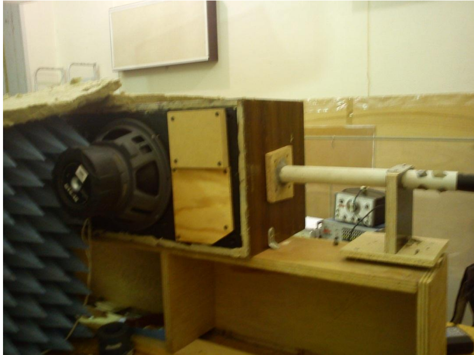
Picture 2: A vacuum cleaner pipe mounted to wooden box with an attached loudspeaker transducer.
