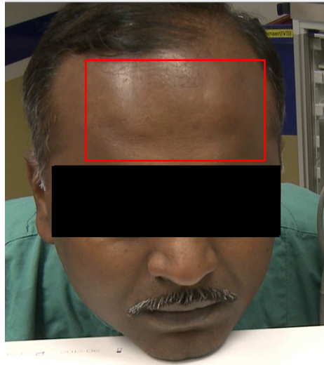
Figure 5.9 – Setup for experiment using PPG to detect HR in darker skin tones. ROI is shown as the red rectangle on the forehead of the subject.
