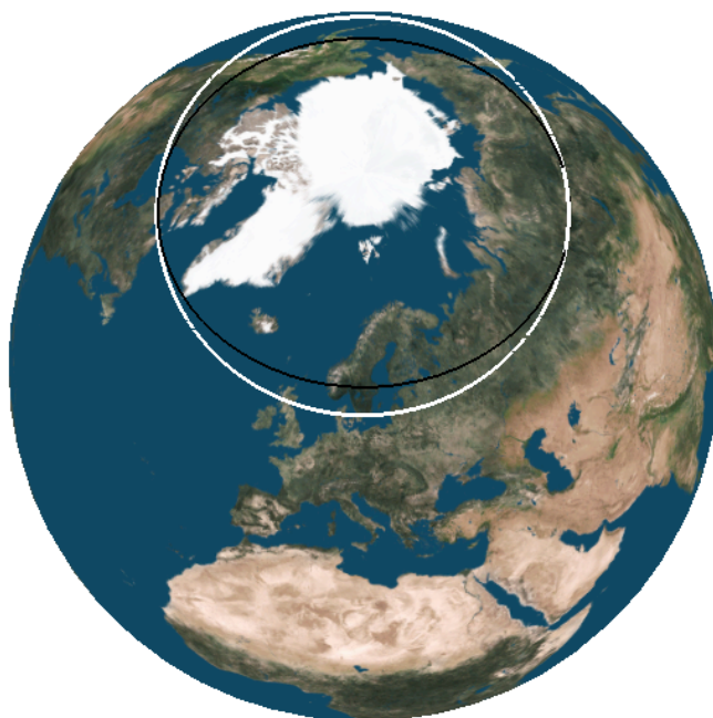
Figure 7.5: Coverage realized by a satellite at apogee with a 9^\circ antenna beamwidth. The black circle show 60^\circ northern latitude, and the white contour indicate the 3 dB beamwidth of a 9^\circ antenna beam.
